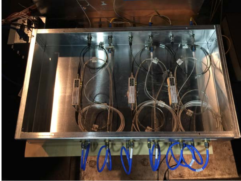
Figure 10. MZM Modules with Inputs (blue RF cables) from the RF Front end
