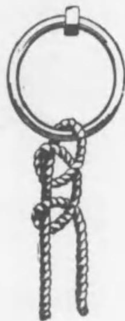
Fig. 3. Two half hitch.
