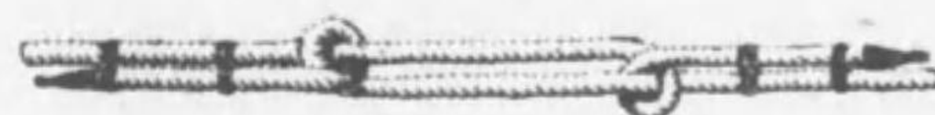
Fig. 9. Reeving line bend.
