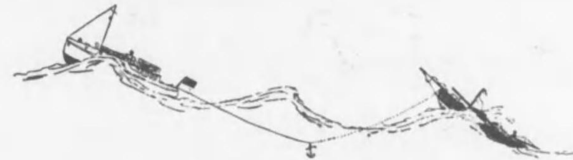
Fig. 2. THE RIGHT WAY. A Weighted Towline of Correct Length.
