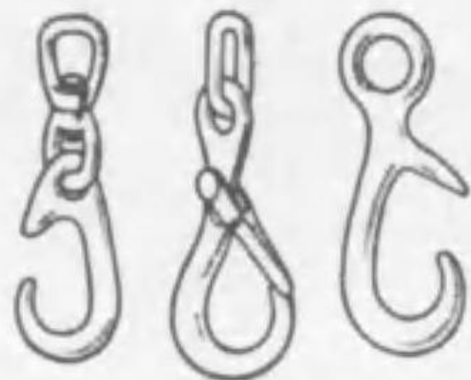
Swivel cargo hook (Liverpool) (hook)
