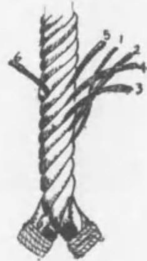
Fig. 8. Wire eye splice.
