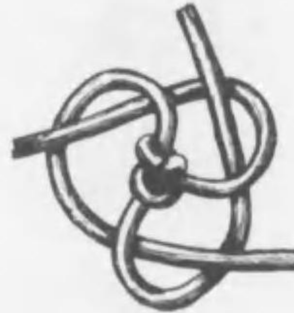
Fig. 9. Single sheet bend.
