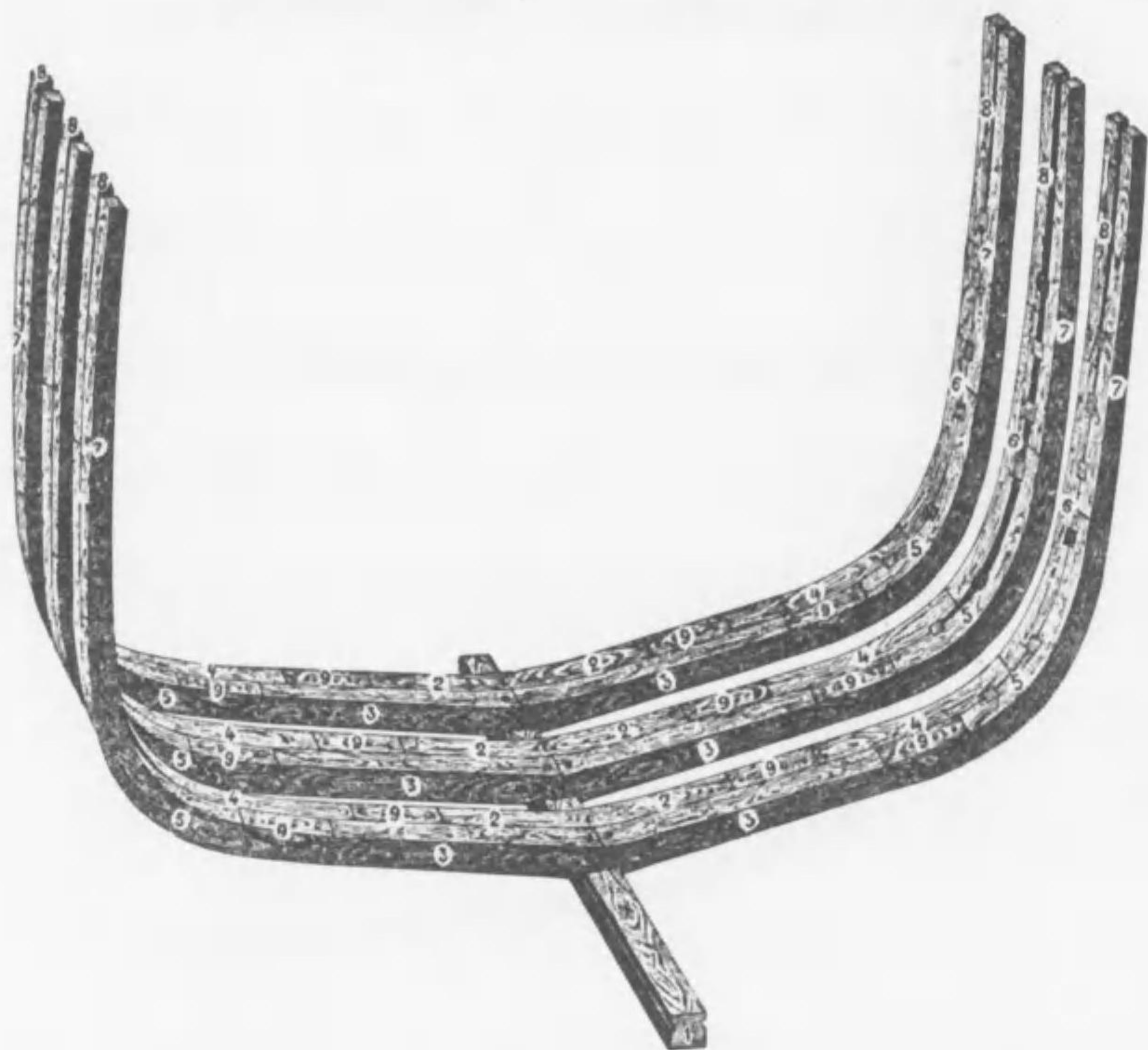
SQUARE-BODY-FRAMES, SHOWING BUTT-CHOCKS, JOINT-DOWELS, ETC. OF A WOODEN VESSEL.
