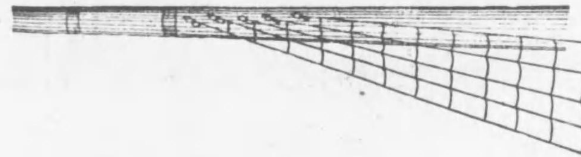
Wire rigging fitted with shackles to masthead.
