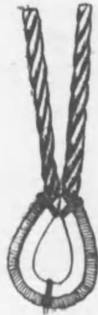
Fig. 2. Wire eye splice.
