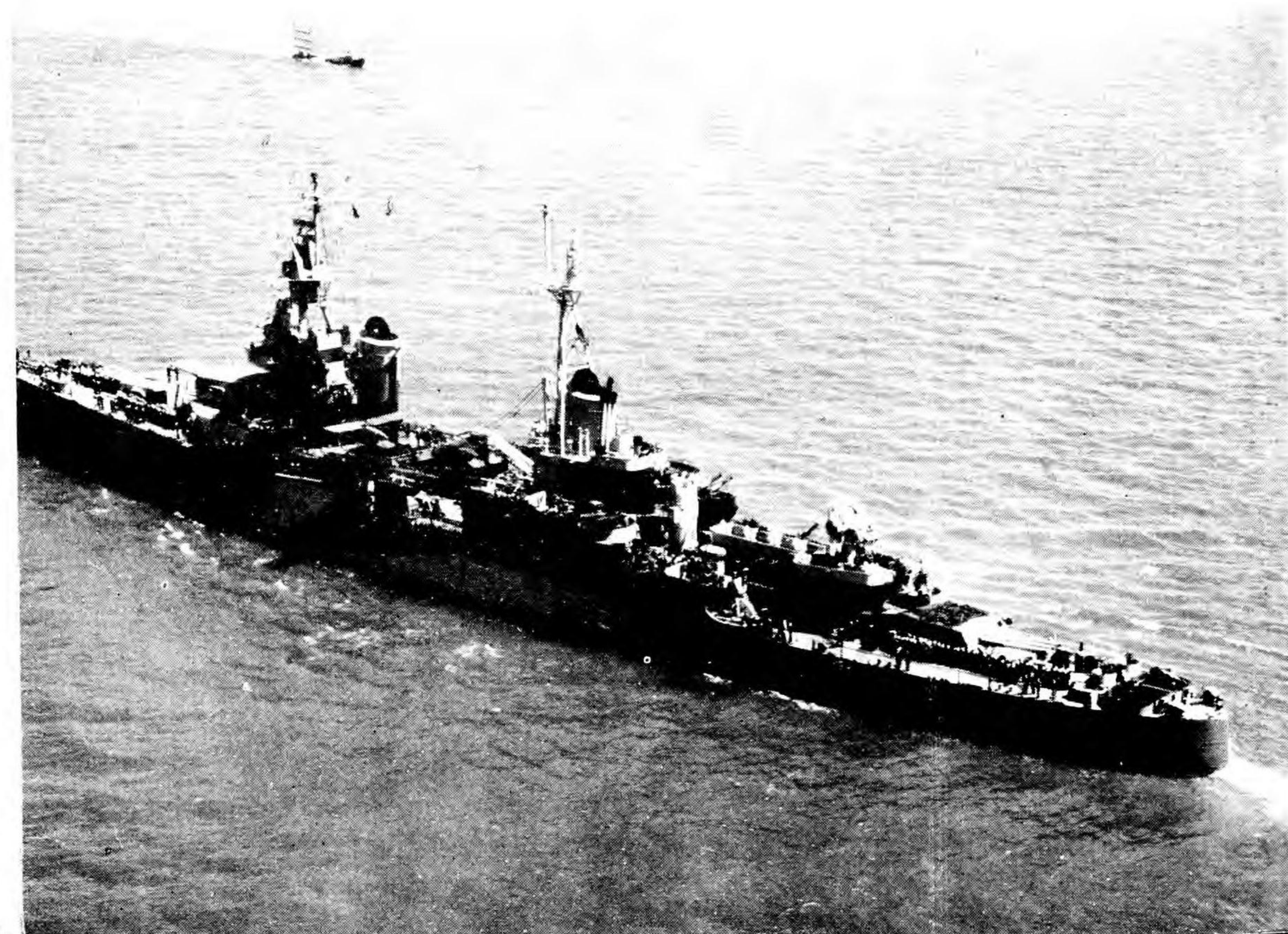
The heavy cruisers Pensacola and Indianapolis (below) after recent alterations. The tripod control tower aft has been removed from the Pensacola . On the Indianapolis , the tripod mainmast has been removed and a new tripod mast has been placed on the after stack, a change planned for all units of the Portland and Northampton classes. (Restricted.)
