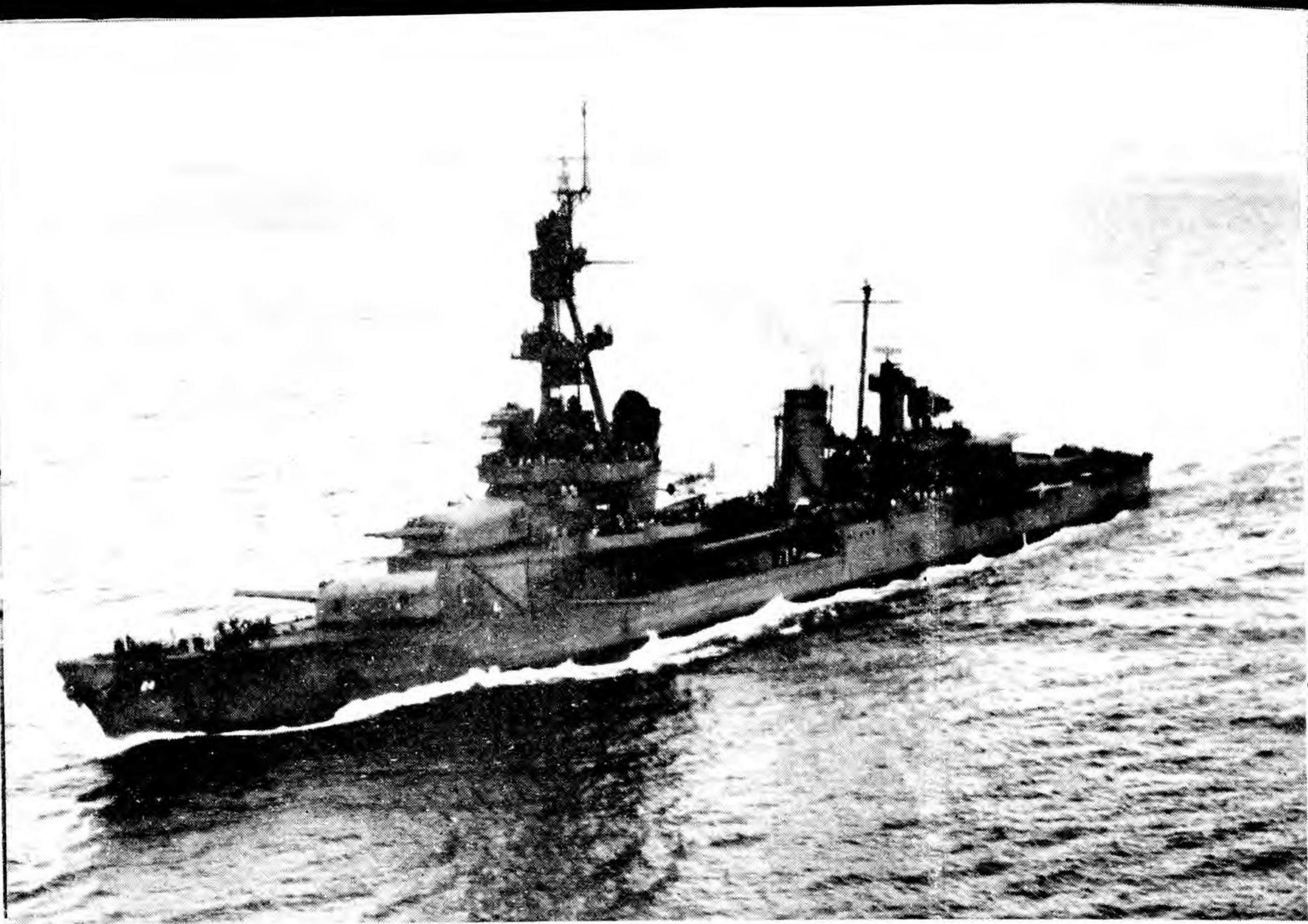
The heavy cruisers Pensacola and Indianapolis (below) after recent alterations. The tripod control tower aft has been removed from the Pensacola . On the Indianapolis , the tripod mainmast has been removed and a new tripod mast has been placed on the after stack, a change planned for all units of the Portland and Northampton classes. (Restricted.)
