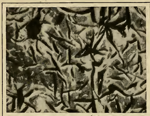
NO. 198. PHOTOMICROGRAPH OF SAND CAST PIG IRON. THE THICK BLACK LINES ARE GRAPHITE FLAKES
