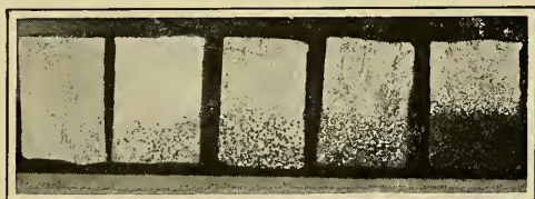
TEST BARS WITH ONE EDGE CAST AGAINST A "CHILL"
