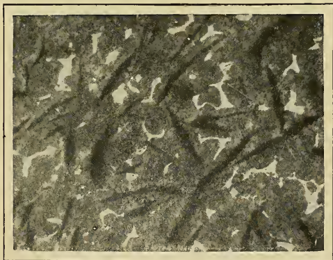
NO. 92d. SEMI-STEEL, A STRONGER GRAY CAST IRON
