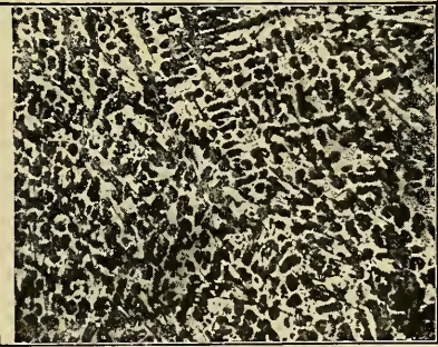
No. 109. WHITE CAST IRON WITH 3 PER CENT CARBON
