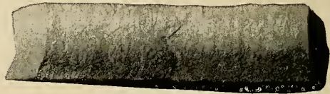
CHILLED CAST IRON
