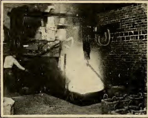
A GRONWALL-DIXON 5-TON ELECTRIC FURNACE TAPPING
