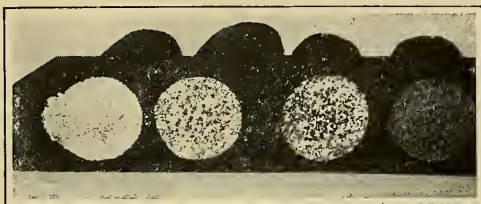
TEST SPRUES, SHOWING WHITE, SLIGHTLY MOTTLED, MEDIUM MOTTLED, AND GRAY FRACTURES
