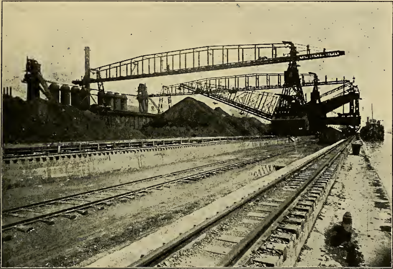
THE REHANDLING BRIDGE WITH STOCK ORE PILE AND BLAST FURNACE AT REAR
