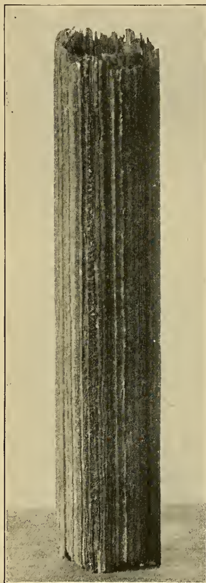
PICKLING IN WEAK ACID EX- POSES THE "FIBERS" OF WROUGHT IRON
