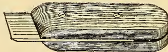
FIG. 116.—Knife for freezing microtome, made from the blade of a carpenter's plane.
