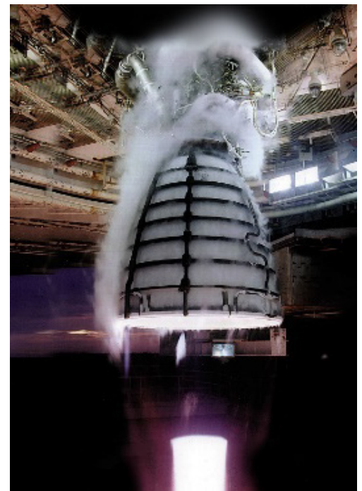
RS-25 engine undergoing a hot-fire test. (NASA)
