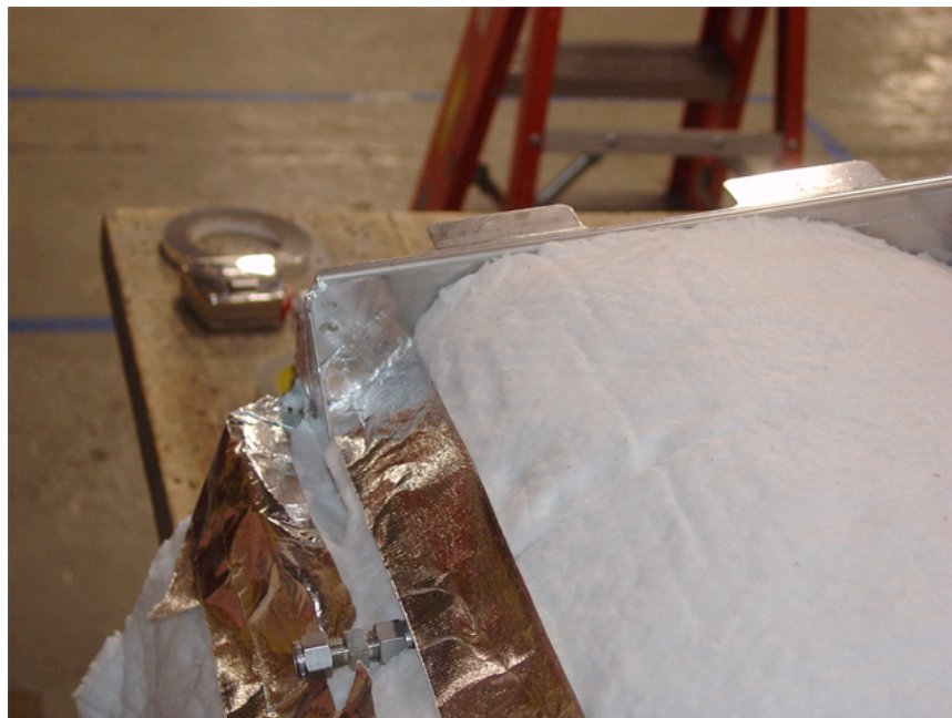
Figure 19. Taping Down the Insulation (Sheet 2 of 2).
