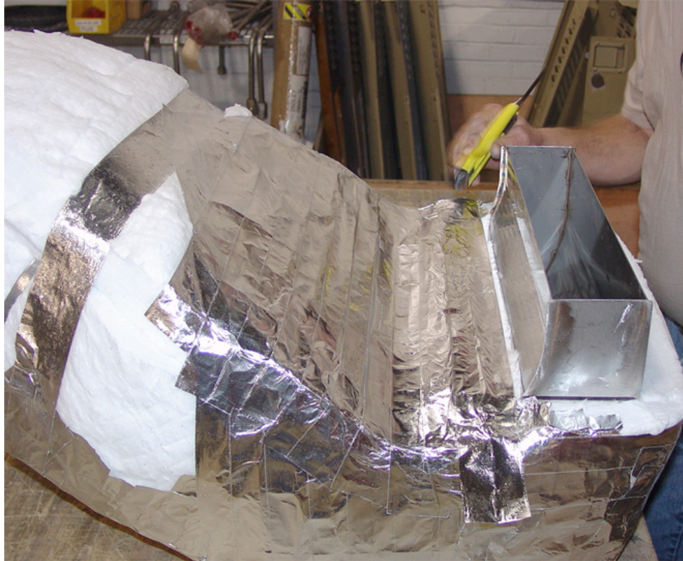
Figure 30. Building the Nonstick Side Around the Plenum Outlet.
