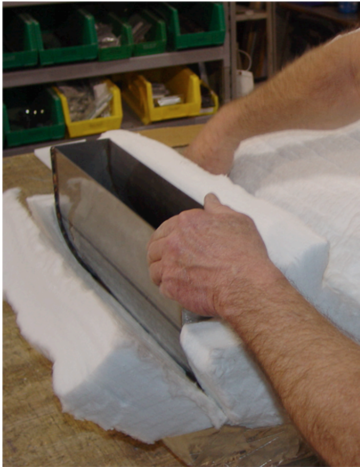
Figure 25. Snugging Insulation into the Bend (Sheet 2 of 2).
