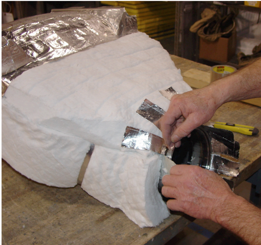
Figure 23. Inlet Tape Cut into Small Slices (Sheet 2 of 2).
