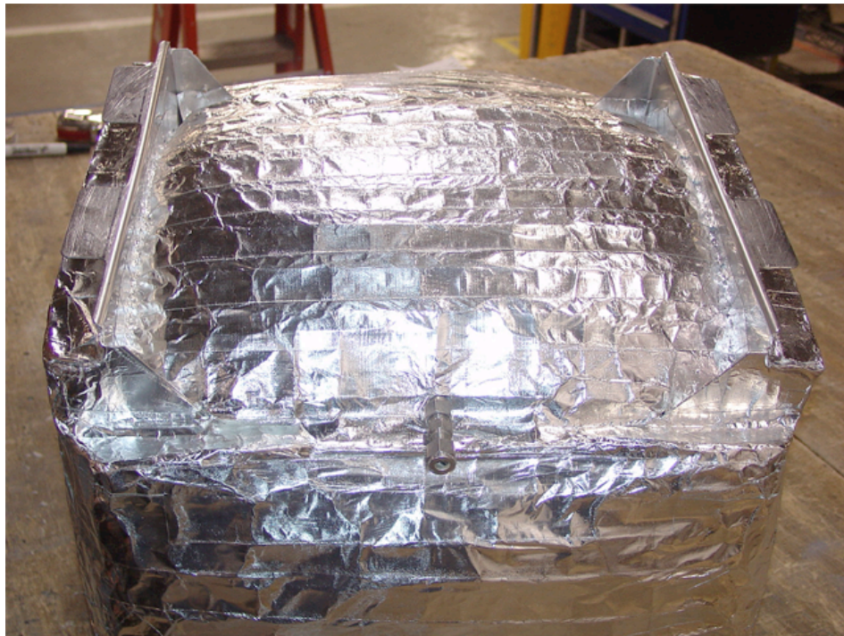
Figure 35. Bottom and Top View of Completed Insulation Wrap (Sheet 1 of 2).
