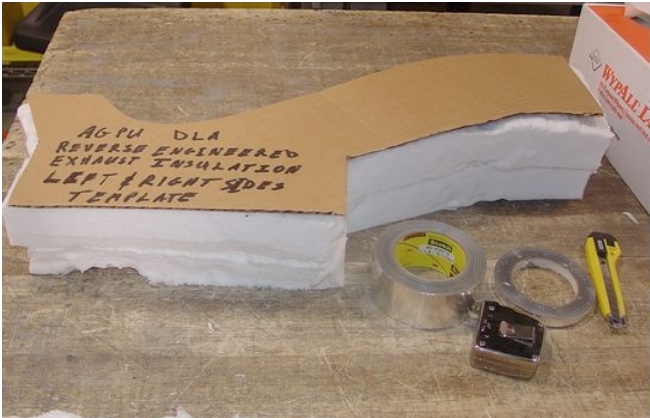
Figure 6. Plenum Template (Sheet 2 of 3).
