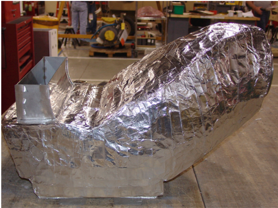
Figure 35. Bottom and Top View of Completed Insulation Wrap (Sheet 2 of 2).
