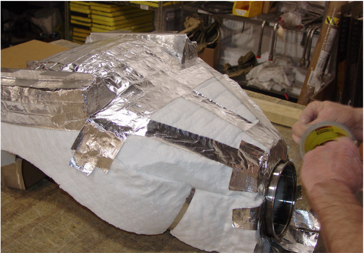
Figure 24. Insulating the Top Snug (Sheet 1 of 2).
