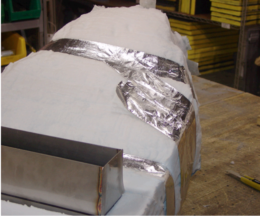
Figure 28. Taping the Top of the Unit (Sheet 1 of 2).
