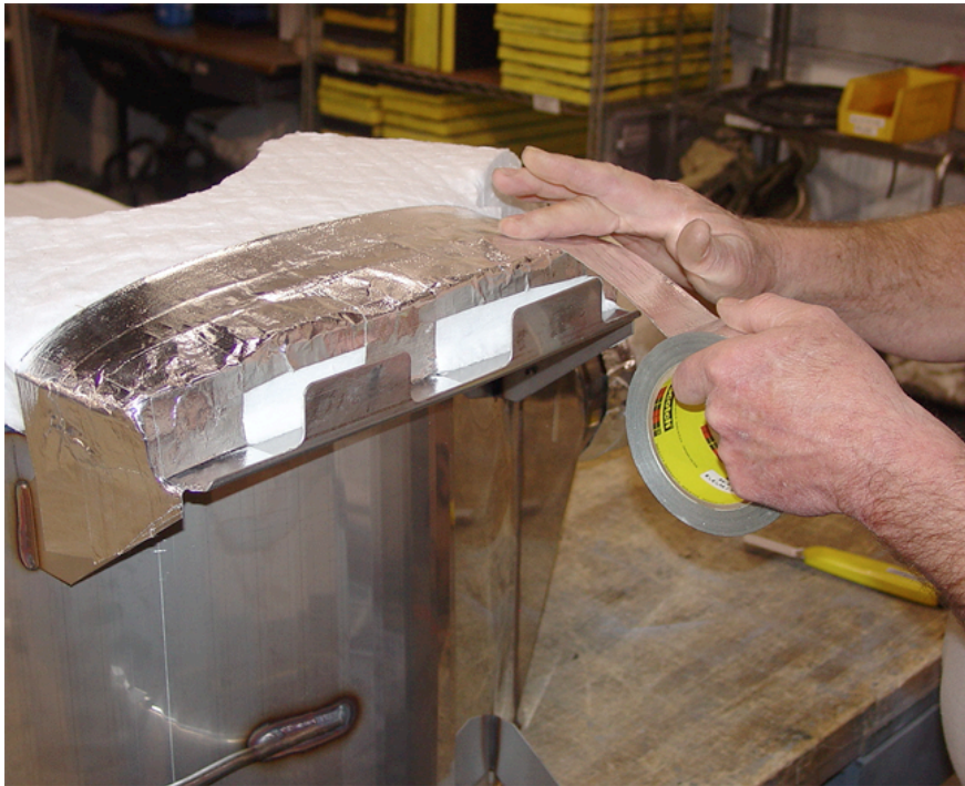
Figure 13. Wrapping of the Plenum.
