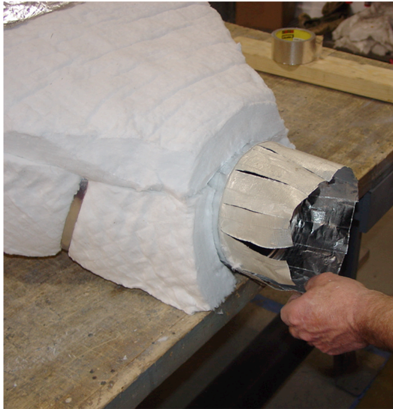
Figure 23. Inlet Tape Cut into Small Slices (Sheet 1 of 2).
