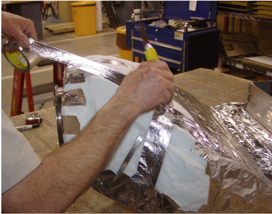
Figure 33. Taping the Top Portion of the Plenum.
