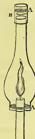
FIG. 5. A glass tube furnished with flame sieves , in which a common candle may be burnt. A A. the flame sieves. B. a little plate of metal to prevent the upper flame sieve from being acted on by the current of hot air.
