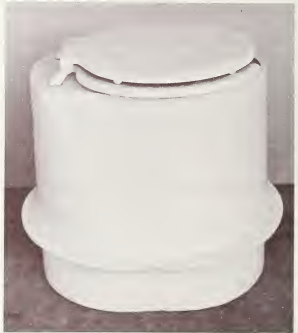
Figure 2. Vault toilet riser fabricated from cross-linked polyethylene.
