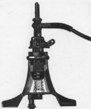
Automatic Stand Showing Position of Parts while being thrown by hand.
