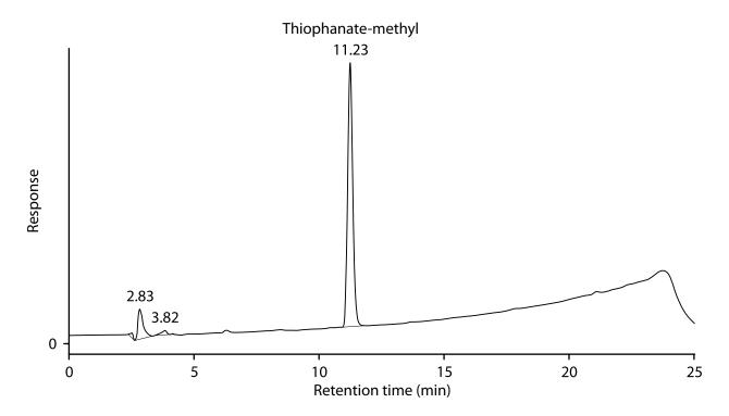
**Figure 1.** This is a typical chromatogram for a sample of thiophanate-methyl. This shows the response for a spike of 348 µg/sample of thiophanate-methyl on an OVS-2 tube, extracted and analyzed by this LC method using the Kingsorb<sup>™</sup> column. On the Synergi<sup>™</sup> column, the retention time for thiophanatemethyl is 14.1 minutes.
