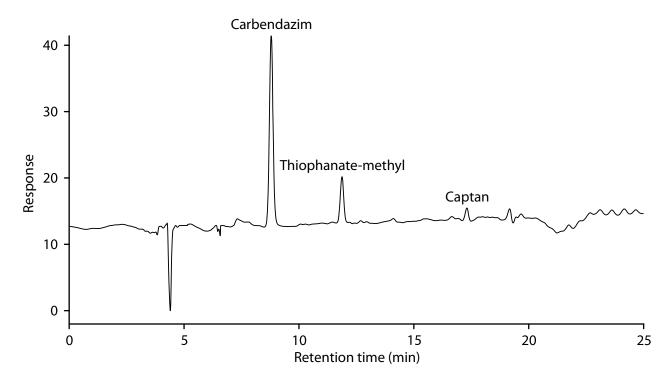
**Figure 3.** This chromatogram shows the three analytes of interest, carbendazim, thiophanate-methyl, and captan, which were extracted from a spiked OVS-2 sampling tube. This chromatogram has been background corrected by subtracting an OVS-2 blank analysis.
