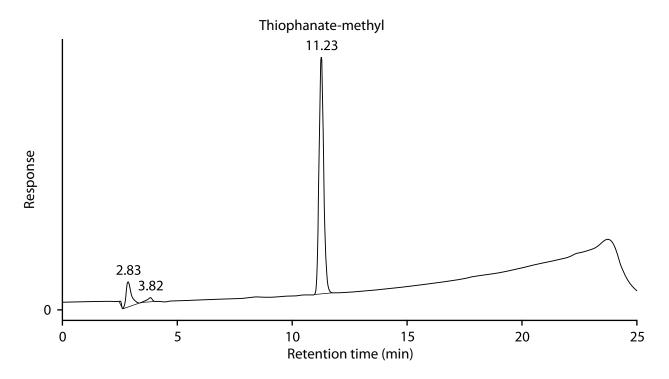
**Figure 2.** This is a typical chromatogram of a liquid calibration standard. This sample was analyzed with the Kingsorb<sup>™</sup> column. The retention time on the Synergi<sup>™</sup> column is 14.1 minutes.
