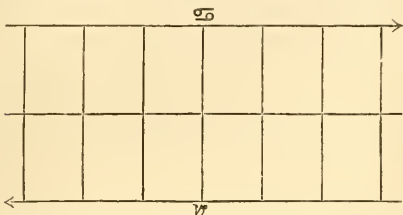
FIG. 51.—Diagram showing how the sun's apparent motion along the ecliptic, now parallel with the earth's equator (the central line of the figure) at the summer ( \odot ) and winter ( \omega ) solstices, is represented by equal intervals along the equator.
