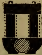
Diagram of magnetic circuit of Edison dynamo. Leakage coefficient 1.4.
