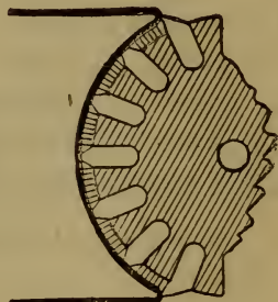
Figure 33 Bunching of magnetic lines in air gap.
