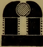
Diagram of magnetic circuit of T. H. bipolar dynamo. Leakage coefficient 1.3.
