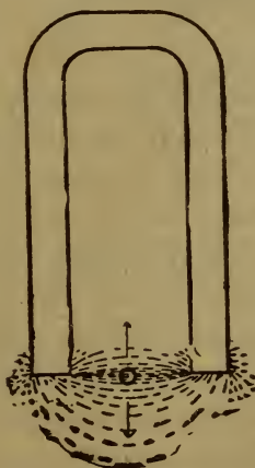
Figure 20 Wire carrying current in a magnetic field tending to move in or out of the magnet.
