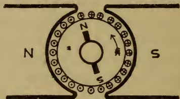
Figure 53 Counter magnetic motive force of armature reaction.
