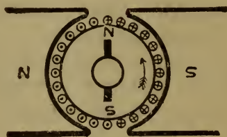
Figure 52 Armature reaction in a dynamo.
