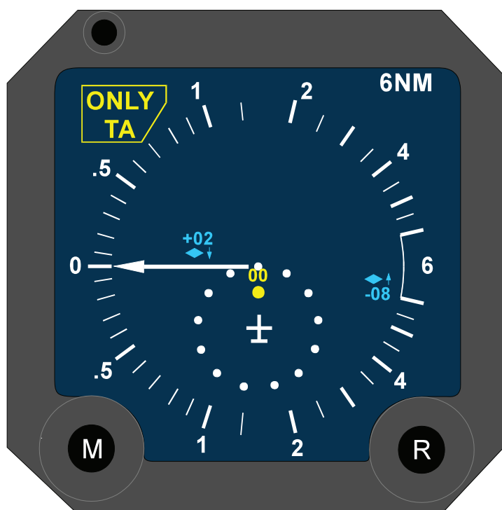
Figure 3B-146. TA ONLY Operational Situation
