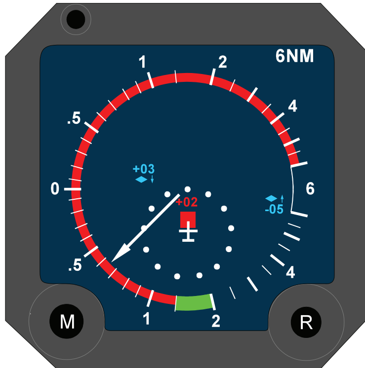
Figure 3B-147. Corrective RA Operational Situation
