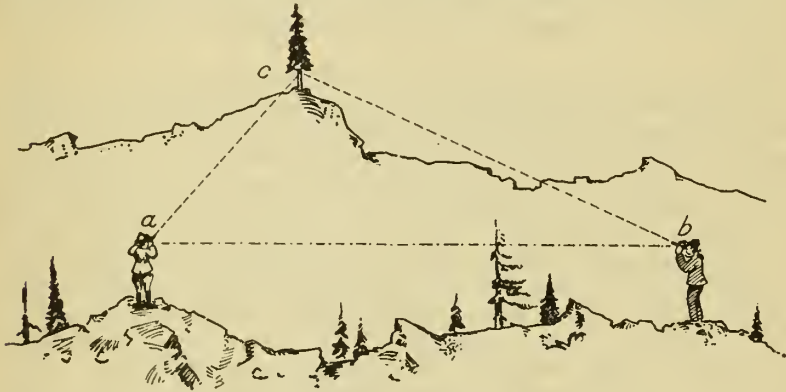
FIG. 27.—Use of Abney on minor triangulations
