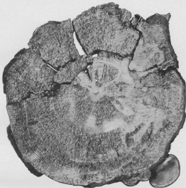
FIG. 1.—CROSS SECTION OF WESTERN HEMLOCK TRUNK, 75 FEET FROM THE GROUND, KILLED BY FIRE FOUR YEARS BEFORE, SHOWING RATE OF DECAY CAUSED BY POLYPORUS PINICOLA.
