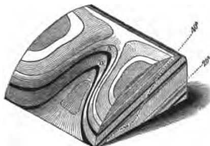
Slope of valley 40°, dip of strata 20°.
