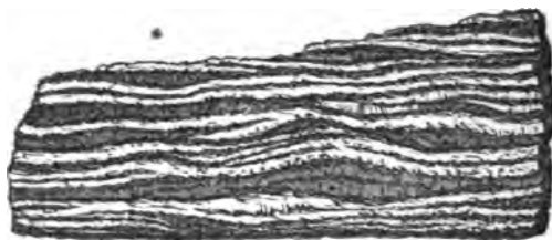
Fragment of gneiss, natural size; section at right angles to planes of stratification.
