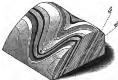
Slope of valley 20°, dip of strata 50°.
