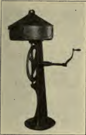
Figure 10.—The Original Babcock Tester. Courtesy of Wis. Exp. Sta.
