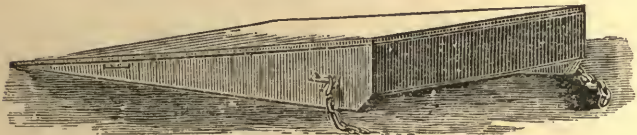
Fig. 5.—PLATFORM FOR DRYING EARTH.
