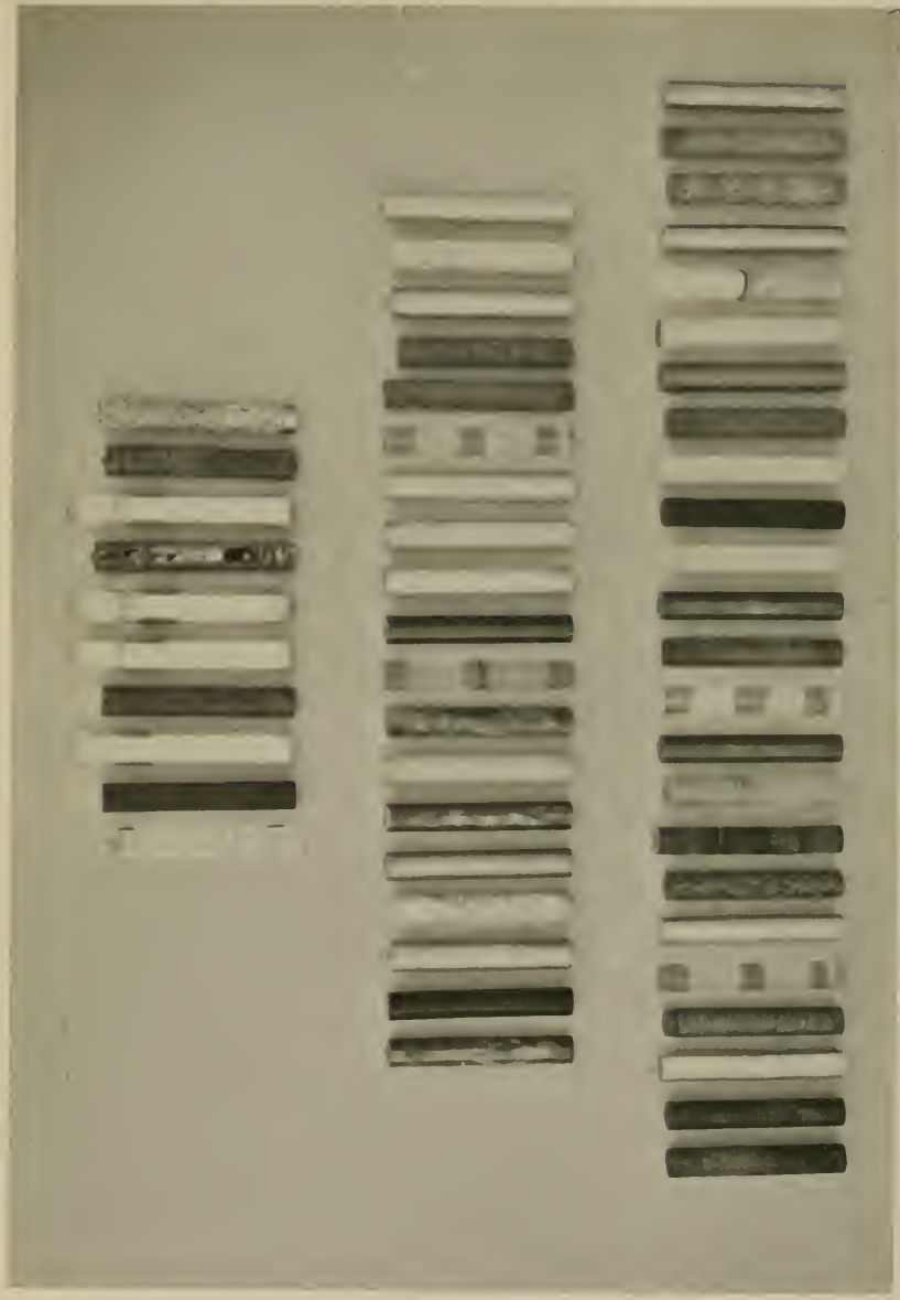
A PORTION OF THE CYLINDRICAL SPECIMENS ON WHICH COMPRESSIBILITY MEASUREMENTS BY THE PISTON-DISPLACEMENT METHOD HAVE BEEN MADE
