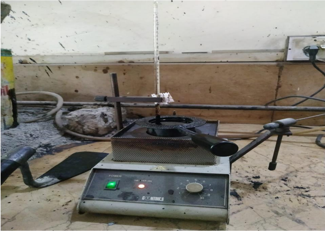
Fig. 7.9: Flash Point and Fire Point Test
