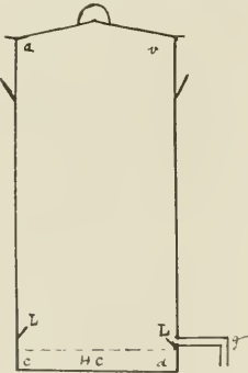
Fig. 2.—Vertical tank still; ab, 12 inches; ac, 28 inches; CL, 4 1/2 inches; LL, 1-inch ledge.
