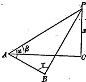
$$\text{又自 } \triangle PAB, \quad PA = \frac{AB \sin \angle PBA}{\sin \angle APB} = \frac{a \sin \gamma}{\sin(\alpha + \gamma)},$$
