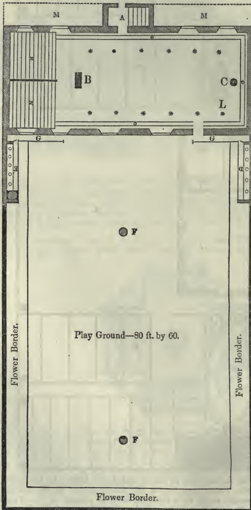
School-room, 60 feet long by 25 feet wide, and 18 feet high.
