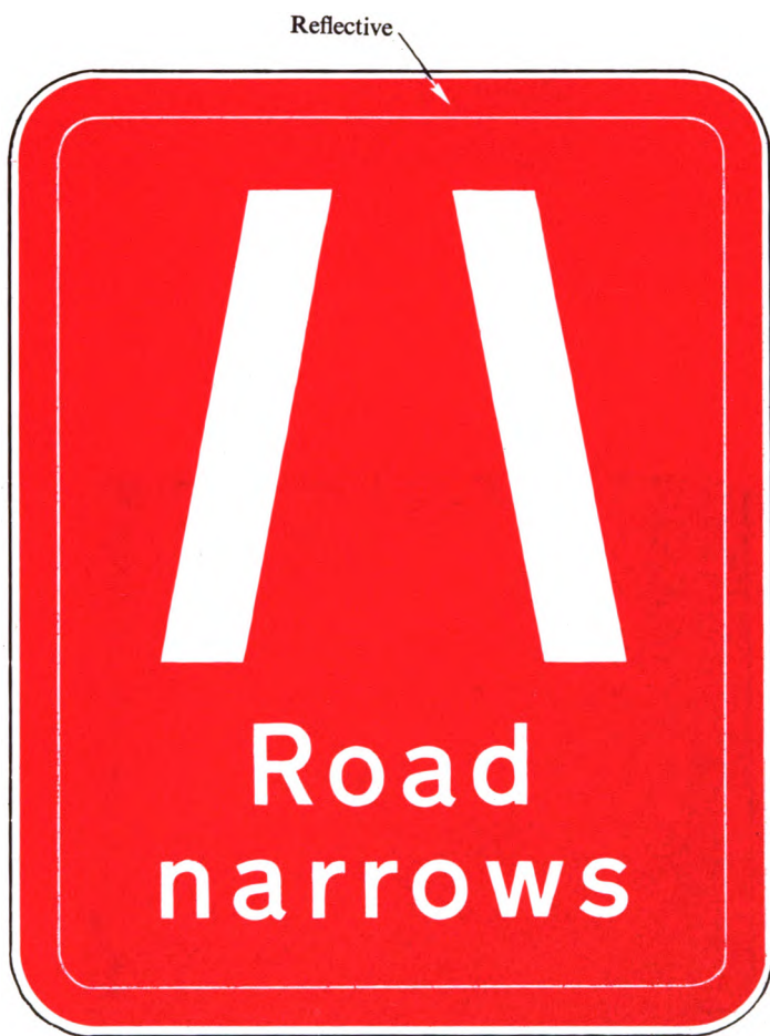
Figure 56. Sign to give warning that the motorway narrows. (Paragraph 145)
