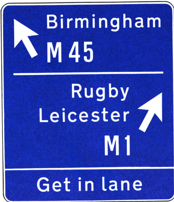
Figure 39. Alternative design for second advance direction sign for a junction of two motorways. (Paragraph 107)
