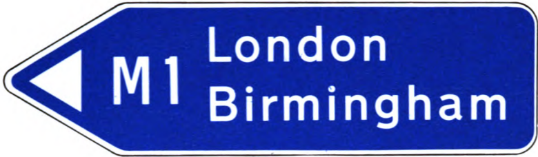
Figure 9. Supplementary sign at a junction with, and indicating, a motorway. (Paragraph 58)
