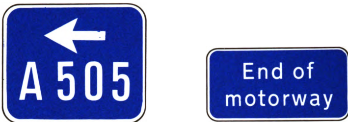
Figure 32. Supplementary exit sign for use where there is not room for place names. (Paragraph 95)
