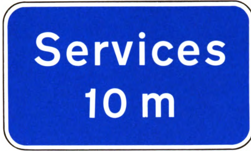
Figure 47. Sign to be erected, where appropriate, after each intersection along the motorway. (Paragraph 136)
