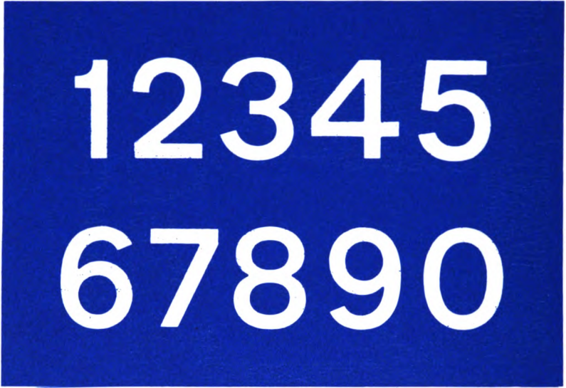
Figure 3. Form and proportion of numerals for all uses except in route-numbers (see figure 4). (Paragraph 15)
