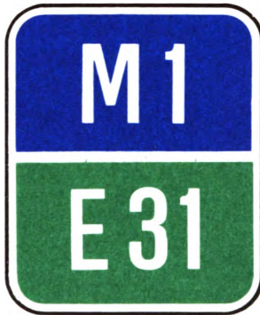
Figure 14. Route-number confirmatory sign on the motorway. (Paragraph 67)
