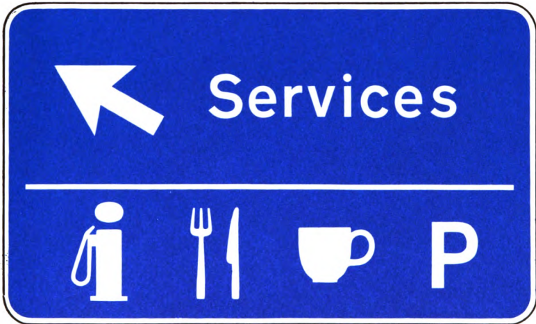
Figure 50. Sign to be erected at the beginning of the deceleration lane leading to a service area. (Paragraph 139)
