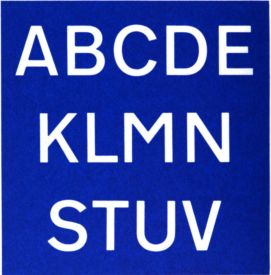
Figure 1. Form and proportion of capital letters, where employed, for all uses except in route-numbers (see figure 4) and telephone numbers (see figure 5). (Paragraph 15)
