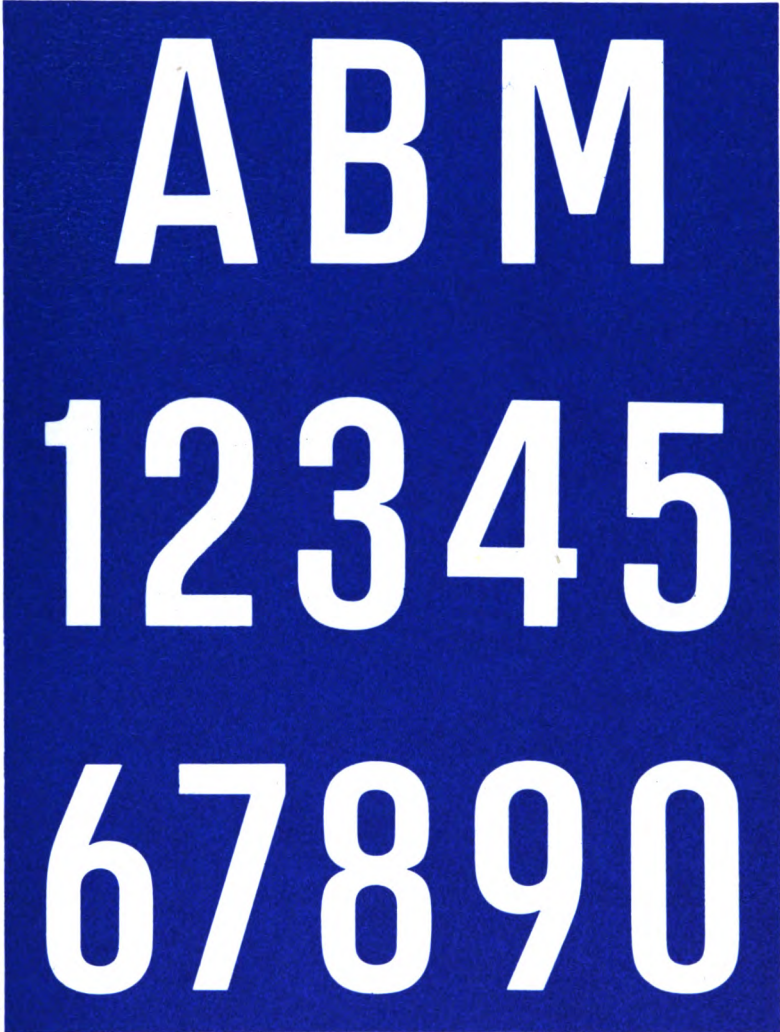
Figure 4. Form and proportion of letters and numerals for use in route-numbers. (Paragraph 15)
