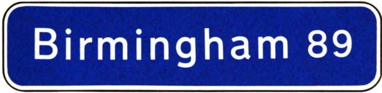
Figure 13. Confirmatory sign on the motorway. (Paragraph 66)
