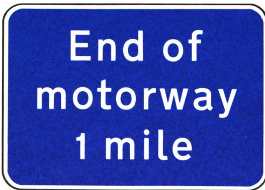
Figure 46. Sign to give warning of approach to end of motorway. (Paragraph 127)
