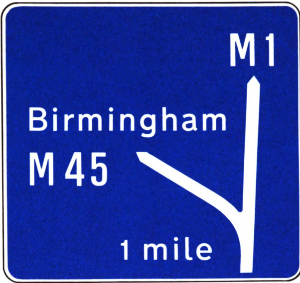
Figure 38. Alternative design for first advance direction sign for a junction of two motorways. (Paragraph 104)
