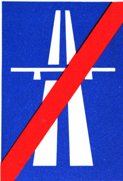
Figure 2. Sign adopted by the Inland Transport Committee of E.C.E. to denote the end of a motorway. (Paragraph 43)
