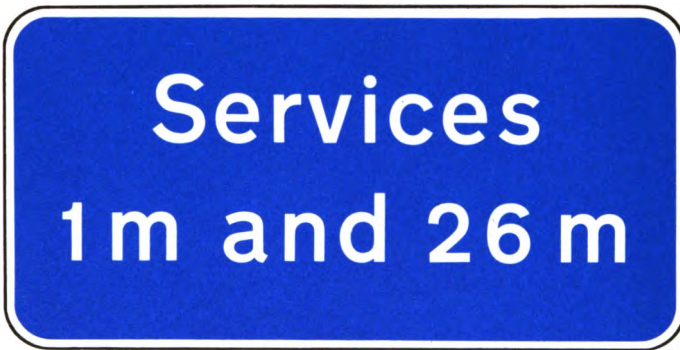
Figure 48. Sign to be erected one mile before the first of two or more service areas along the motorway. (Paragraph 137)
