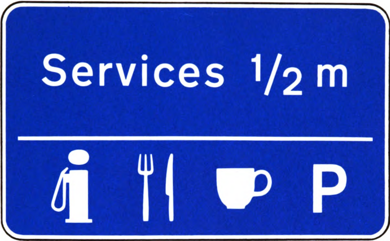
Figure 49. Sign to be erected half a mile in advance of a service area. (Paragraph 138)
