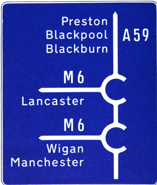
Figure 7. Advance direction sign on the immediate approach to a junction with the motorway which incorporates two roundabouts. (Paragraph 57)
