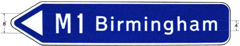
Figure 8. Supplementary sign at a junction with, and indicating, a motorway. (Paragraph 58)
