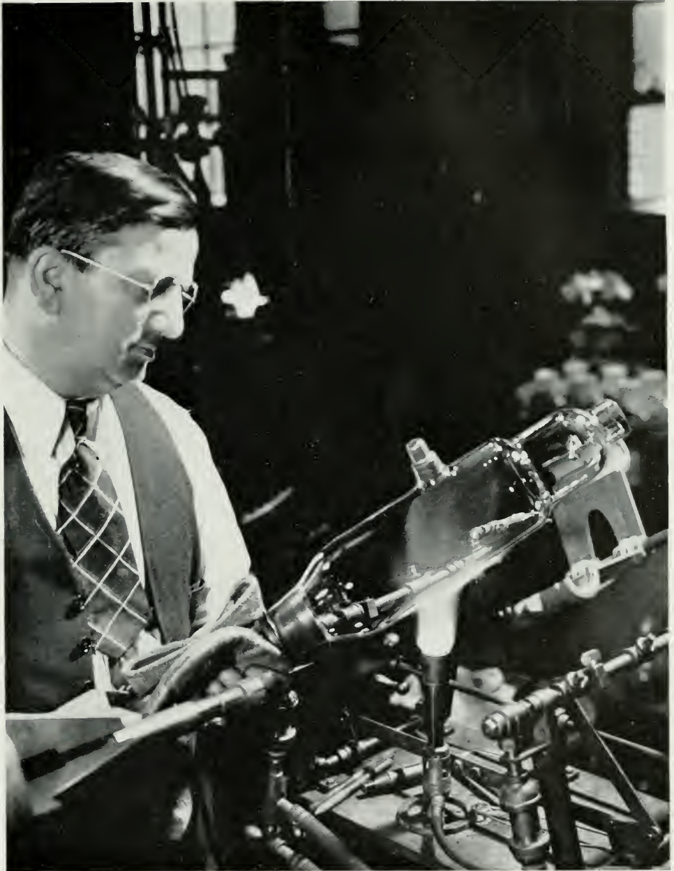
Flame from the bunsen burner plays upon the glass envelope of a vacuum tube, preventing too rapid cooling after the glass has been sealed. Under the watchful eye of the expert, the tube is gently nursed to keep it from cracking.
