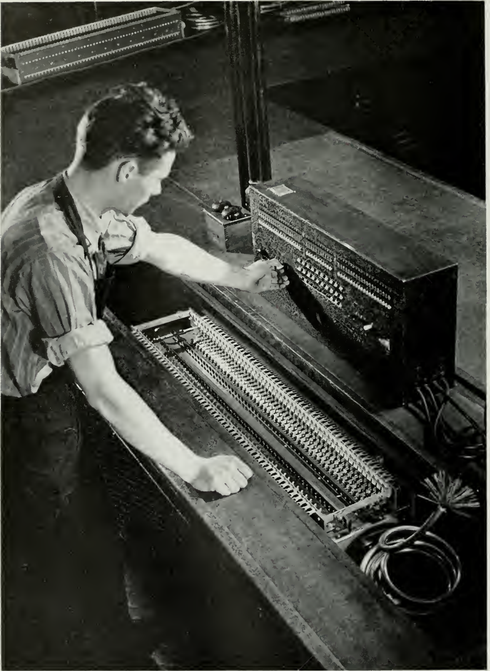
This set tests 204 connections on a cable terminal. Placed upon the elevator in the set, the cable terminal is lowered until it makes the proper contacts within the set. By throwing a switch on the panel, the operator starts a sequence of electrical tests which show up defects in insulation or wiring.
