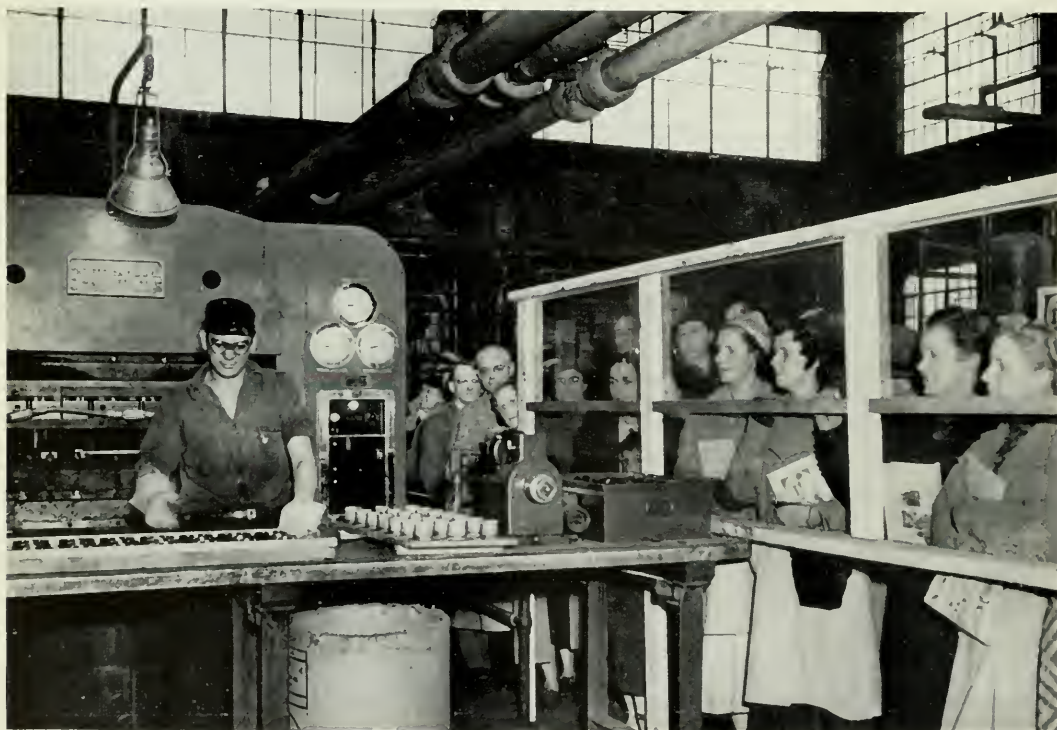
WATCHING PHENOL PLASTIC PASSES WHICH TRANSFORM DUST-LIKE RESINS INTO GLOSSY TELEPHONE PARTS THROUGH HEAT AND PRESSURE. NOTE THE GUIDE BOOKS IN VISITORS' HANDS
