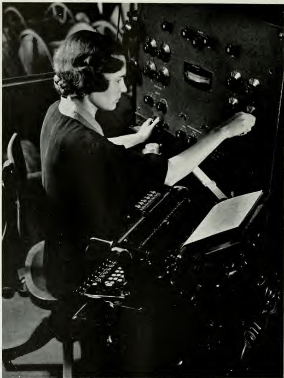
Detecting what the human eye cannot observe—the electrical values of telephone cable. This testing equipment determines whether the resistance and capacitance of representative pairs of conductors meet their specified requirements.
