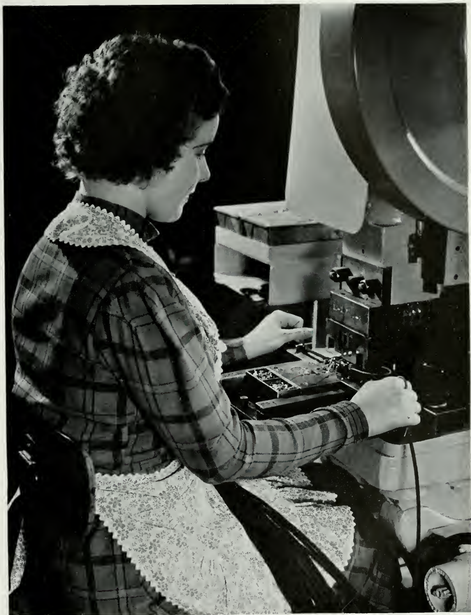
Telephone cords get their finishing touches. The punch press operator is putting terminals and metal supporting bands on the cords.
