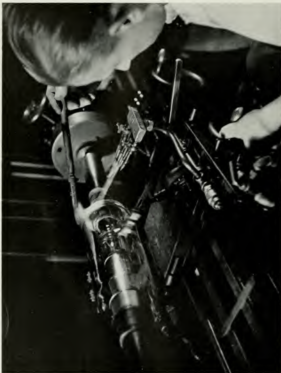
Mounted on a device similar to a lathe, the glass tube and the copper band spin swiftly before the gas flame and finally form a perfectly sealed joint. Thus a water-cooled type of transmitting tube gets its copper collar.
