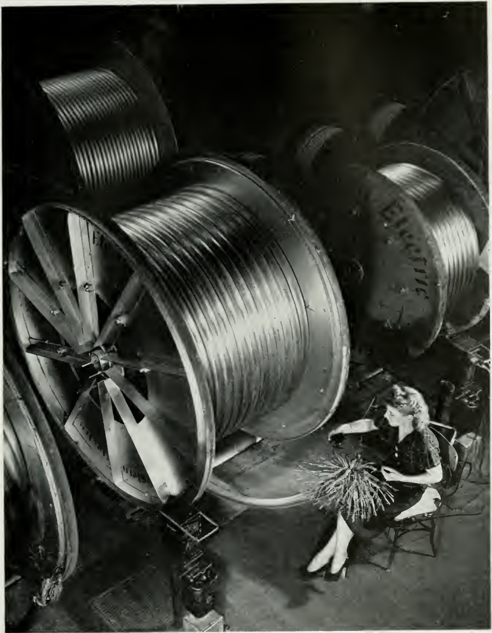
Before being sealed and shipped from the factory, this large toll cable is inspected for electrical properties, which are important for proper transmission of telephone messages. The inspector here connects one pair of conductors at a time to leads from the testing apparatus, enabling another inspector located a short distance away to make the necessary measurements.
