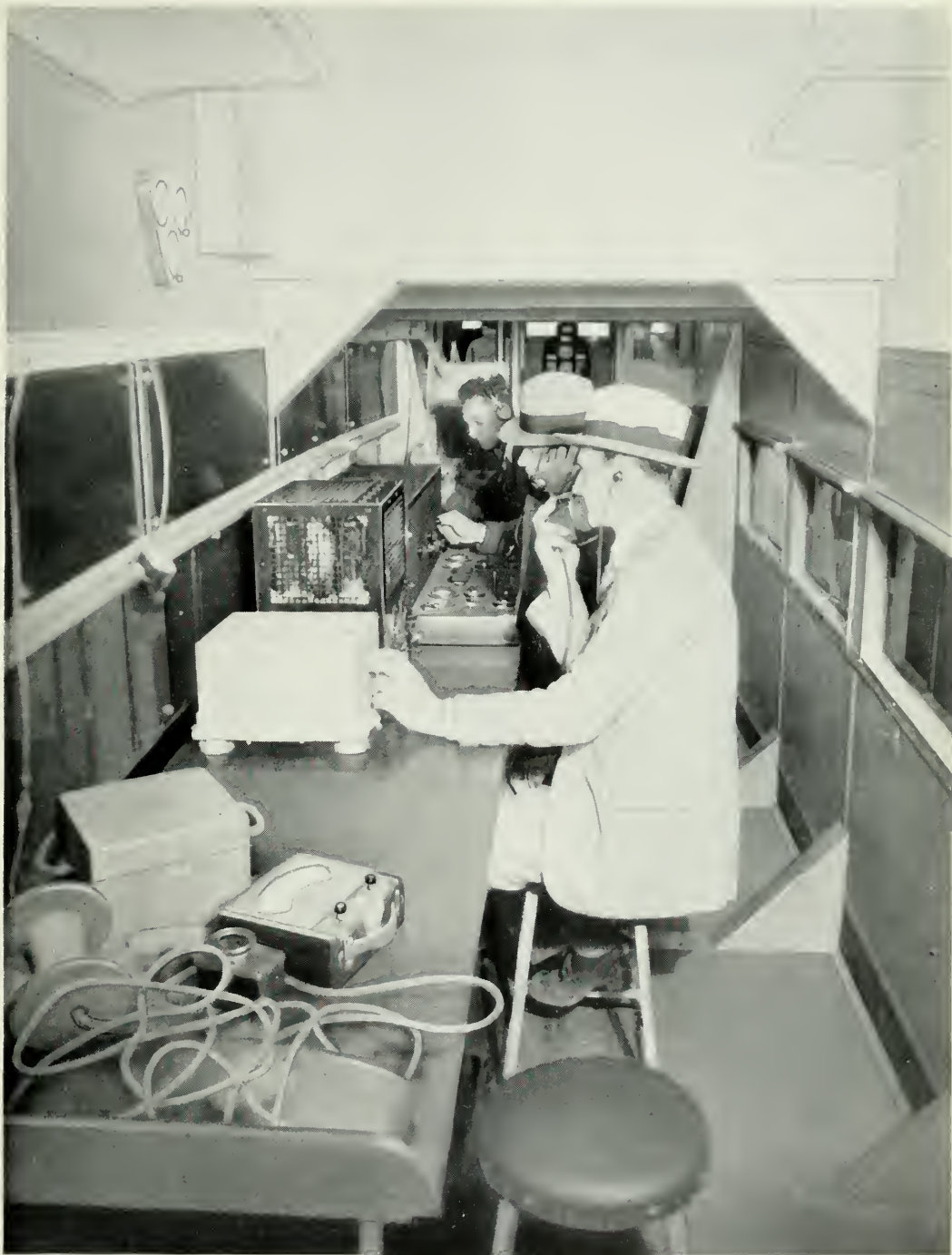
LITERALLY A LABORATORY IN THE AIR: THE INTERIOR OF THE FORD PLANE DURING EARLY TESTS (IN 1929), SHOWING THE LABORATORIES' FIRST MODERN RECEIVER AND TRANSMITTER IN OPERATION IN THE FOREGROUND, WHILE MEASUREMENTS OF FIELD STRENGTH OF THE ASSOCIATED GROUND STATION ARE IN PROGRESS BEYOND. THE PILOT AND CO-PILOT ARE JUST VISIBLE AT THE CONTROLS.
