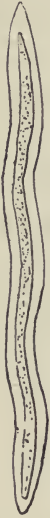
FIG. 116.—A wood fiber, consisting of a much elongated cell with thick woody walls.
