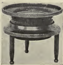
FIG. 72.—A cheap magnifier well adapted for use in analyzing seeds. The magnifier is set over the seeds, leaving the hands free to separate the seeds as one looks through the magnifier from above.
