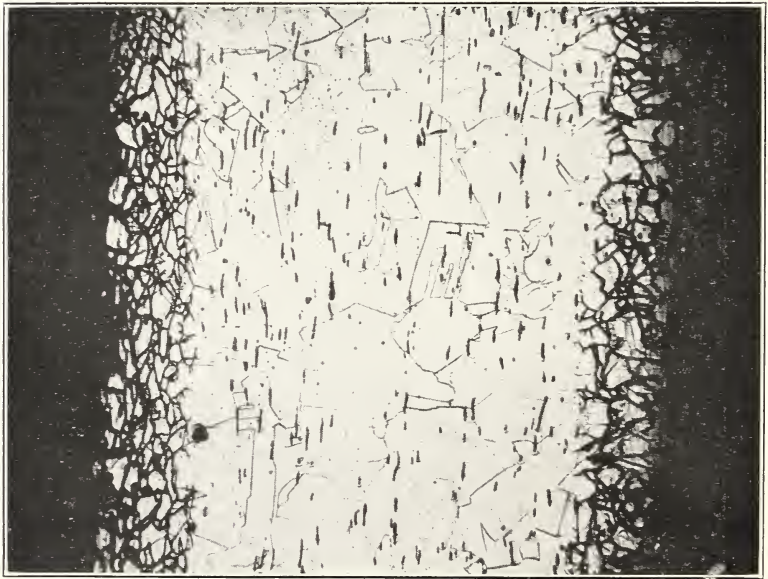
FIG. 4.—Microstructure of cross section of heat-checked nickel sheet, showing intercrystalline oxidation of surface layers. \times 100
