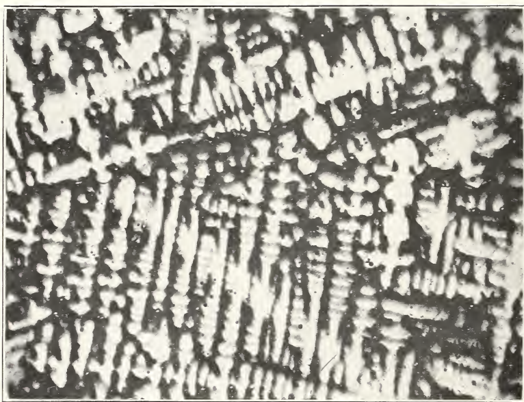
FIG. 13.—Microstructure of cast Monel metal. \times 100
