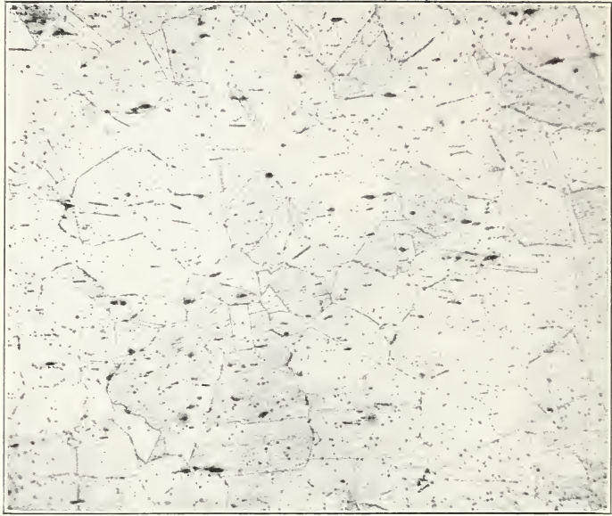
FIG. 3.—Microstructure of rolled nickel rod containing precipitated graphite in the form of fine particles. \times 100
