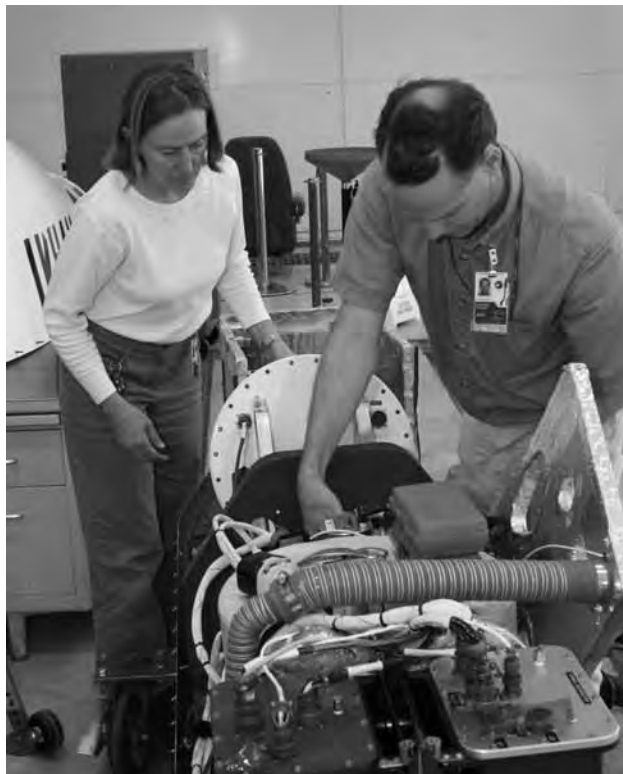
NASA Ames engineers Sally Buechel and Ted Hildum prepare to load the Autonomous Modular Scanner into the Ikhana unmanned aircraft's payload pod.
