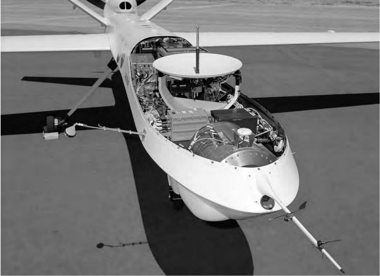
A Ku-band satellite communications system provided the Altair with uplink/downlink capabilities for beyond-line-of-sight control by a pilot in a ground station.
