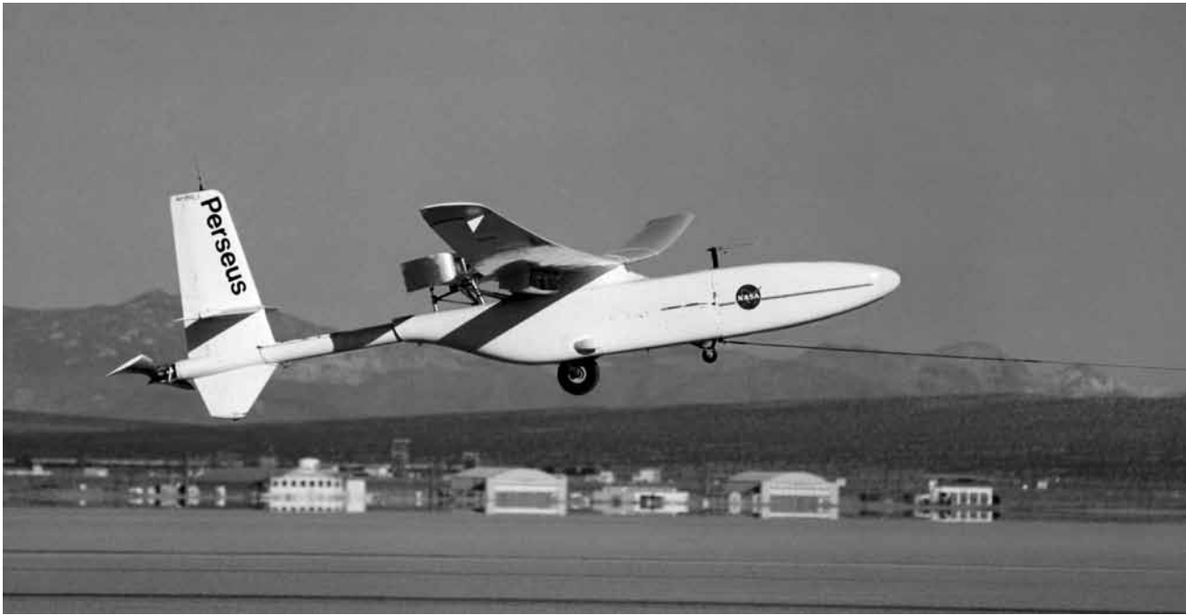
Perseus-A, a remotely piloted, high-altitude research vehicle designed by Aurora Flight Sciences Corp., was towed aloft by a ground vehicle and its engine started after it became airborne. The airplane reached an altitude of 50,000 feet on its third test flight. NASA
