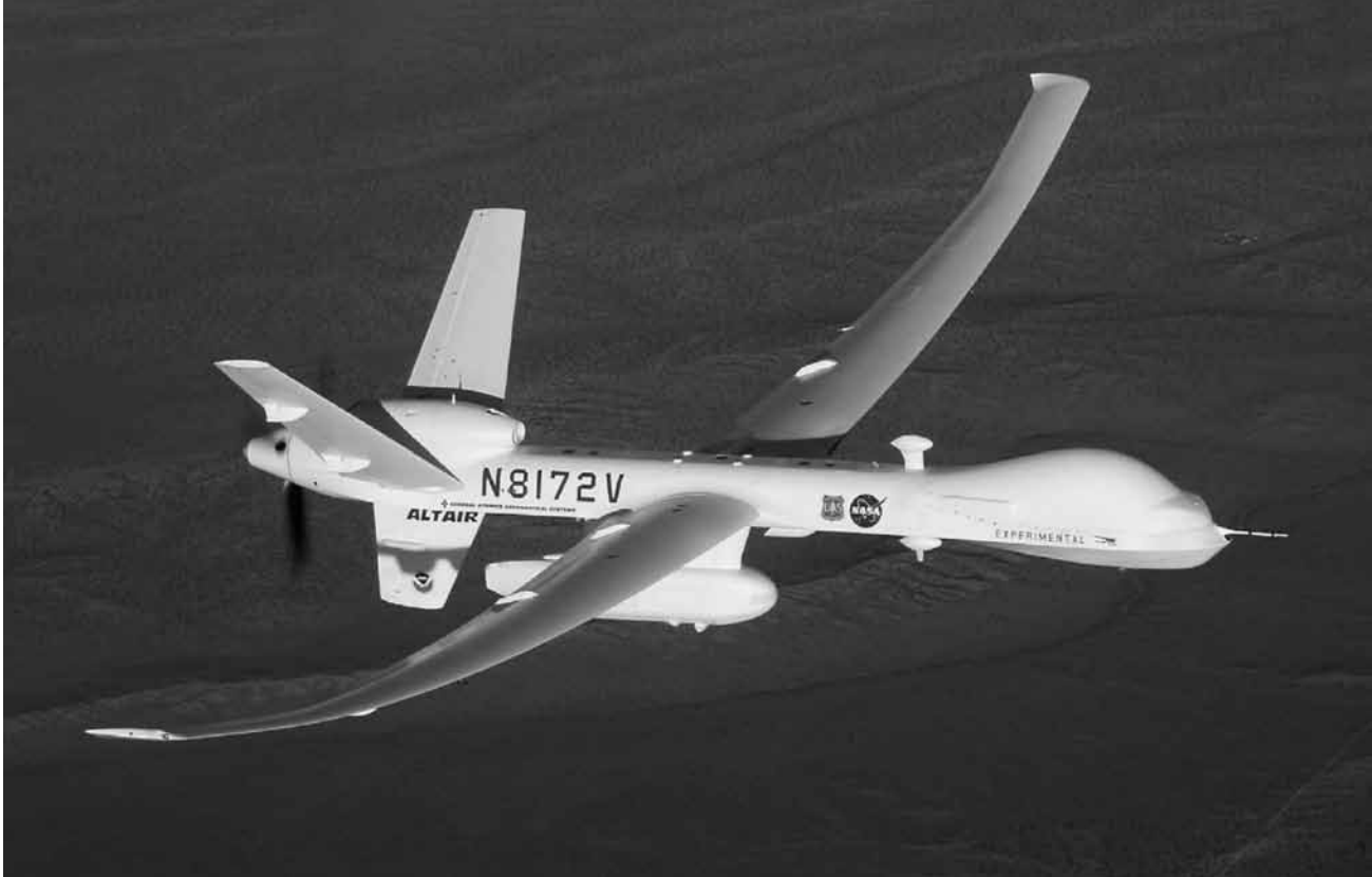
Equipped with a pod-mounted infrared-imaging sensor, the Altair UAS aided fire-mapping efforts over wildfires in central and southern California in late 2006.
