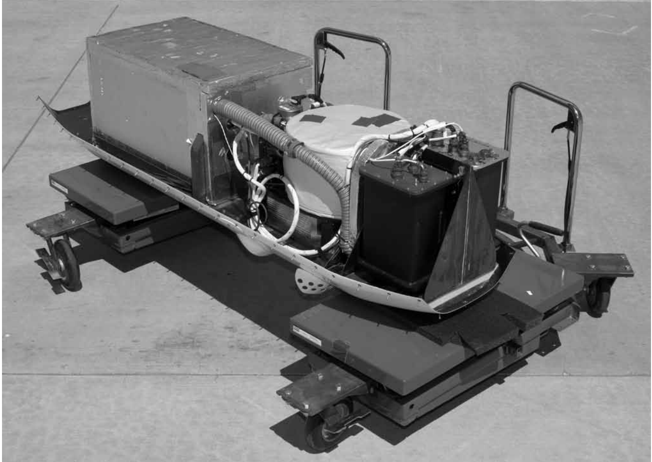
Instruments that make up the Autonomous Modular Scanner include data system computers, scan-head, precision navigation subsystem, power distributor, and control systems.
