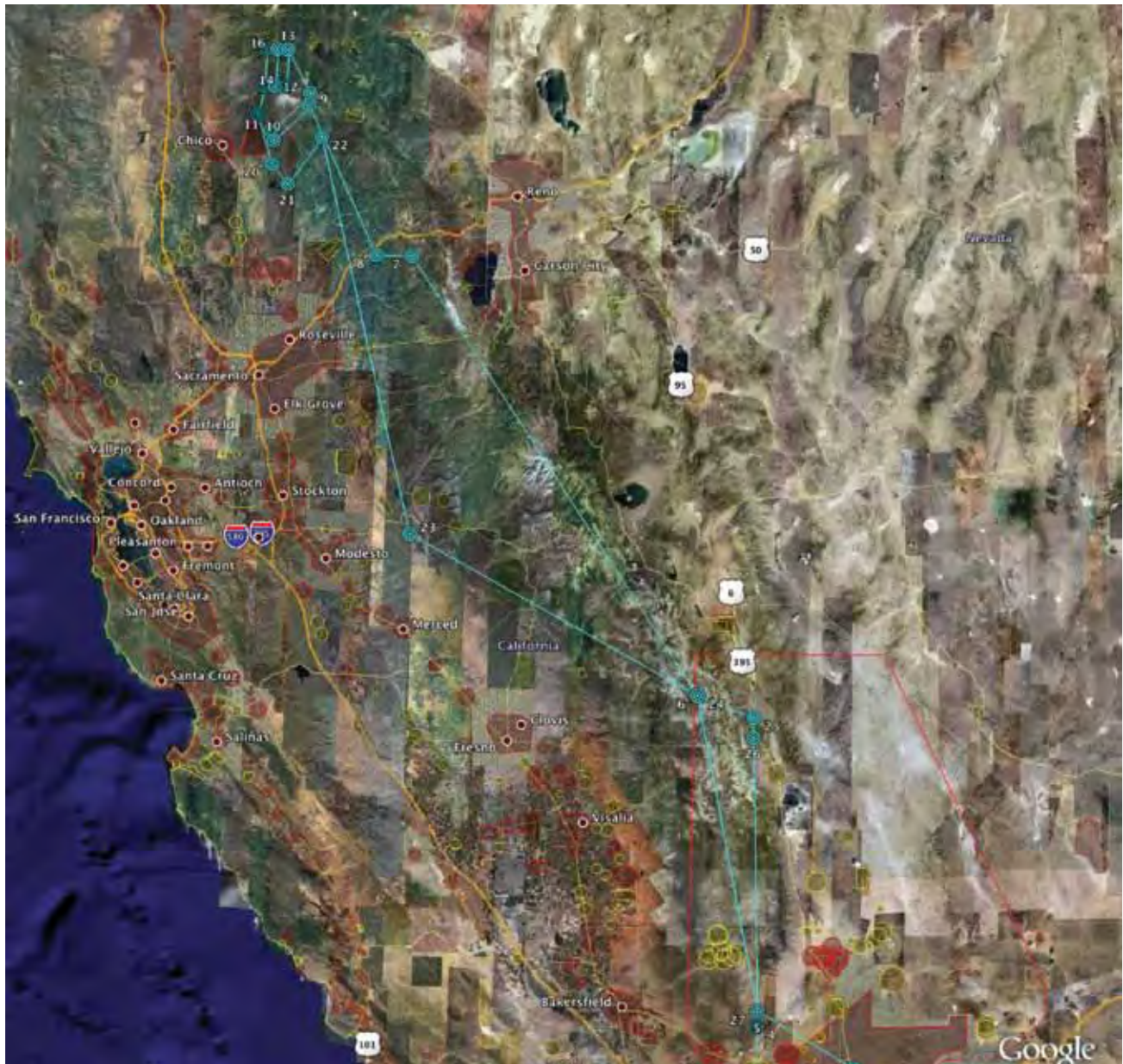
A flight plan for the second WFSM sortie of 2008 shows the aircraft's route over the Sierra Nevada mountain range. Keep-out areas are indicated in yellow and red.
