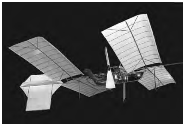
In May 1896, Dr. Samuel Pierpont Langley's steam-powered Aerodrome No. 5 made the world's first successful flight of an unpiloted, engine-driven, heavier-than-air craft. It was launched from a spring-actuated catapult mounted on top of a houseboat on the Potomac River near Quantico, Virginia. The airplane is displayed at the Smithsonian Institution's National Air and Space Museum in Washington, D.C. Courtesy of Brian Nicklas
