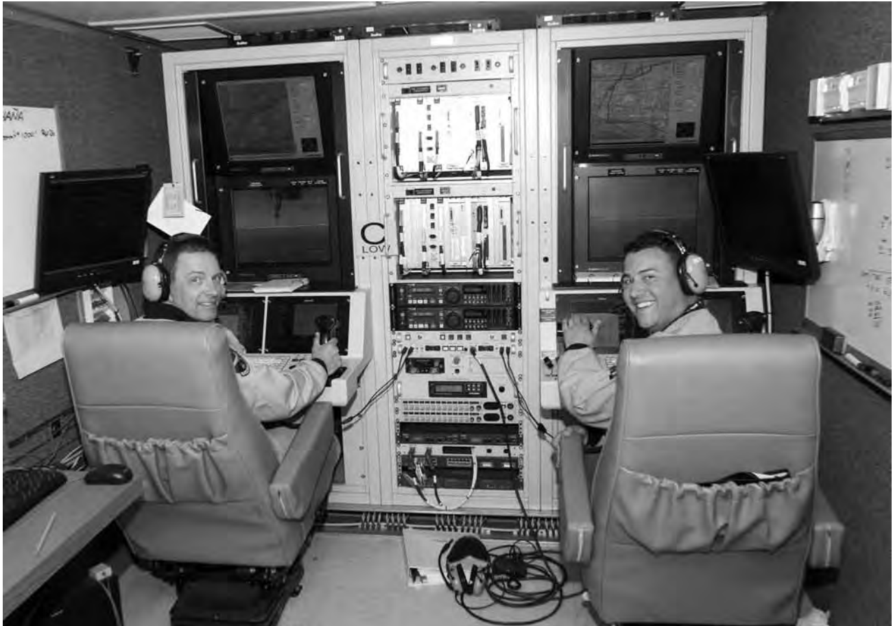
Herman Posada, right, and Mark Pestana seated in the GCS pilot's stations. One pilot flies the aircraft while the other assists with communications and checklists, and serves as a relief pilot when necessary.
