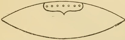
Fig. 127.—Marking Lace-holes on Football Case.
