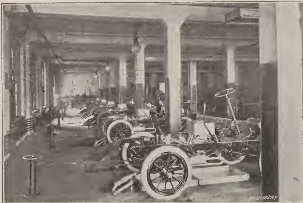
Fig. 6. The Single-cylinder Chassis Testing Stand, arranged for Fan and Brake Resistance
