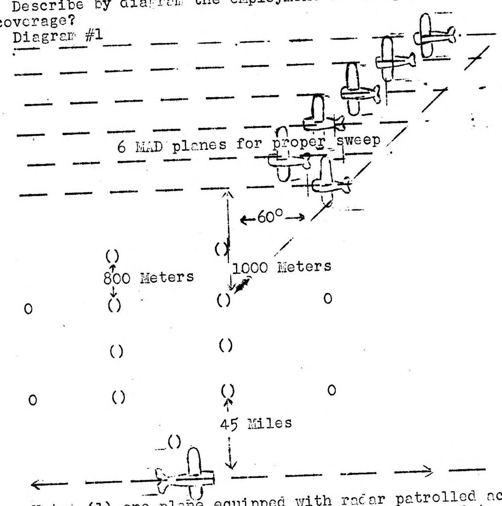
Note: (1) one plane equipped with radar patrolled across stern at distance of 45 miles. This plane was assumed to give radar coverage to 90 miles astern of convoy.
