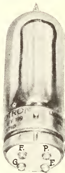
FIG. 3 Showing arrangement of contacts on the UV-199
