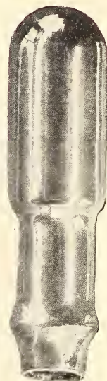
FIG. 5 The glass blank as it is received from the glass factory
