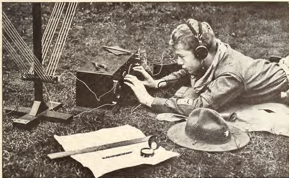
LOCAL RECEPTION ON A LARGE LOOP ANTENNA
