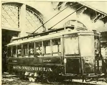
CAR EQUIPPED WITH WESTINGHOUSE ELECTRIC BRAKE AND HEATER SYSTEM FOR DOUBLE TROLLEY OVERHEAD RETURN OR SINGLE TROLLEY GROUND RETURN—RAILWAY EXHIBIT.
