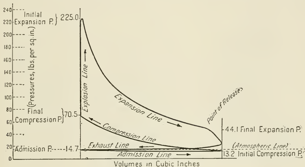
Fig. 2. Indicator Diagram Four-Cycle Engine.
