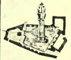
The Ground Platt of Cross Bath at high water holds 52 Tuns 3 Hog. 10 Gall.
