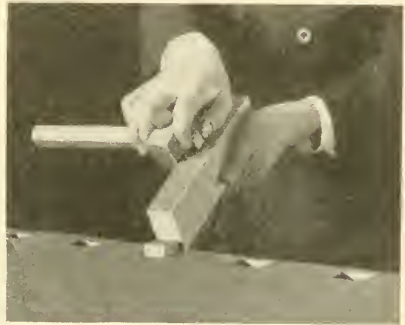
Fig. 5. The Marking Gauge in Use.
