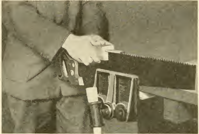
Fig. 24. Jointing a Saw.
