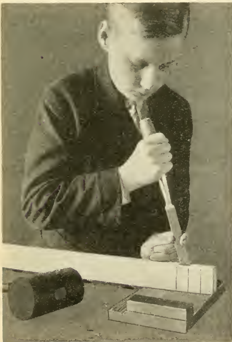
Fig. 20. Method for Holding Chisel in Mortising.
