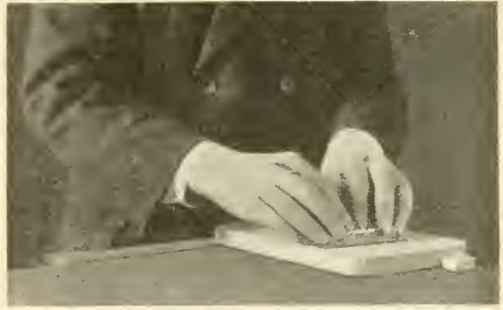
Fig. 11. Position to Hold Sand Paper and Sand Block.
