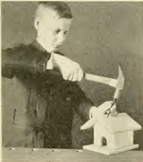
Fig. 18. Setting Nail with Nail Set.
