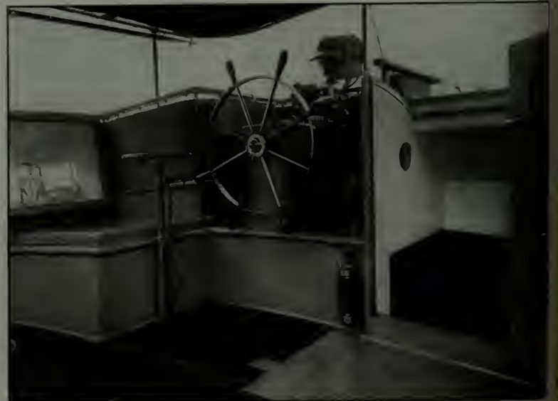
Clever bridge detail arrangement making for one-man control of boat and engine
