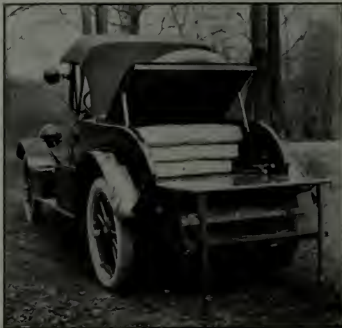
Rear of the car showing construction of the bed frame, which slides out from the floor of the car and is supported in place by folding legs
