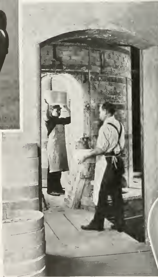
PLACING THE WARE IN THE KILN FOR FIRING, AT THE ROOKWOOD POTTERY
