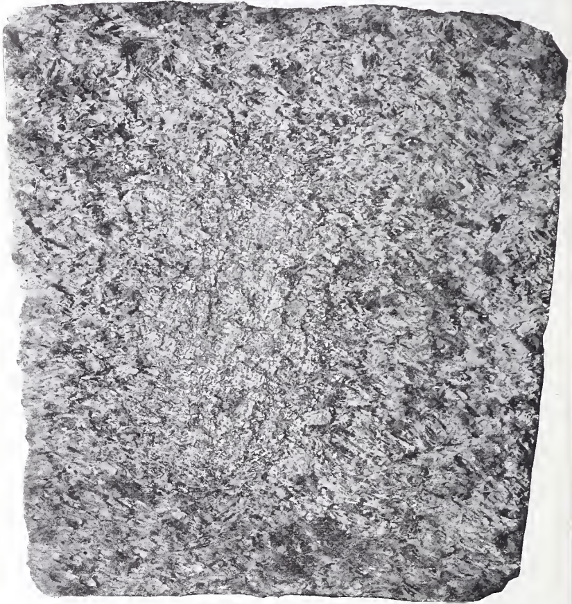
FIG. 34.—Cross section of a block sawed out of a crucible wall containing 90% Ceylon and 10% Pennsylvania flake, also shown in cross section in Fig. 25, and subjected to a temperature of approximately 1250^{\circ}\text{C} in a muffle furnace for 7\frac{1}{2} hours. ( \times 3 .)
