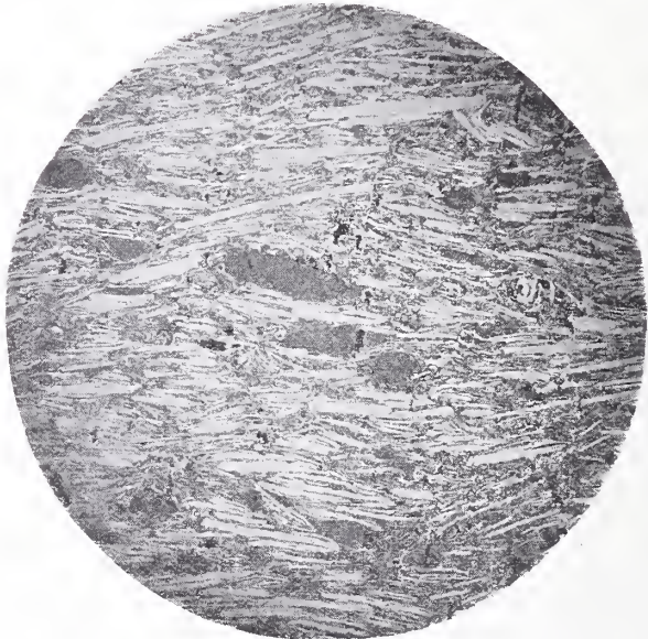
FIG. 18.—Cross section of a portion of a crucible wall in which the graphite is all Madagascar flake, \times 13.3 .
