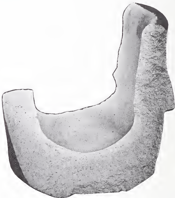
FIG. 4.—Photograph of a section of a chlorinated pot showing depth of penetration.
