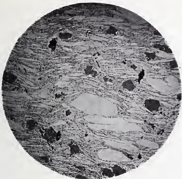
FIG. 27.—Cross section of a portion of a crucible wall said to contain a total of 51% graphite, 75% of which is Ceylon and 25% domestic flake, \times 13.3
