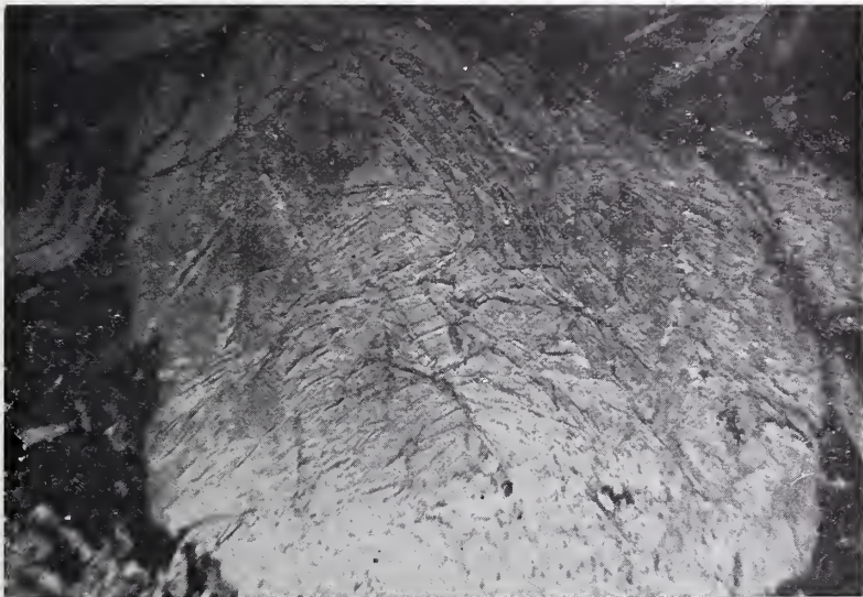
FIG. 12.—Cross section of Ceylon graphite grains embedded in clay, magnified 133 diameters.
