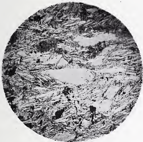
FIG. 28.—Cross section of a portion of a crucible wall, in which 83.5% of the total graphite is reported to be Ceylon and 17.5% domestic flake, \times 13.3 .
