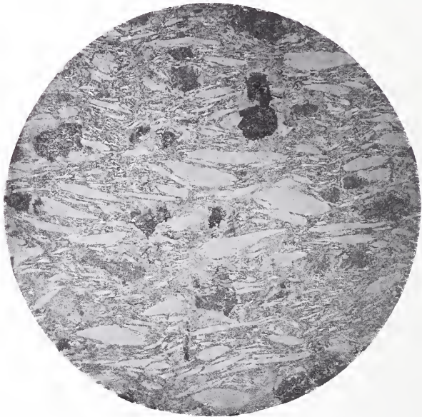
FIG. 22.—Cross section of a portion of a crucible wall in which the graphite is all Ceylon, \times 13.3 .
