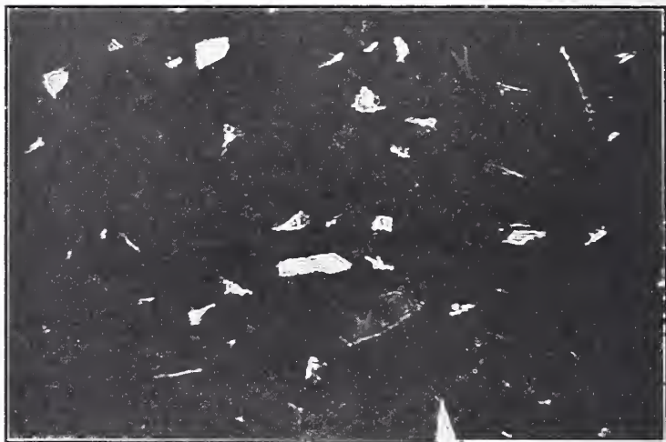
FIG. 9.—The same field as shown in Fig. 5 but taken with crossed nicols. Magnification 300 diameters.
