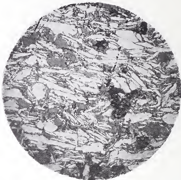
FIG. 25.—Cross section of a portion of a crucible wall in which 90% of the total graphite is Ceylon and 10% Pennsylvania flake, \times 13.3 .
