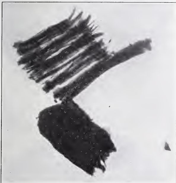
FIG. 14.—Two groups of graphitic oxide plates at a higher magnification. In the one the plates are seen edgewise and in the other flatwise, \times 66 .
