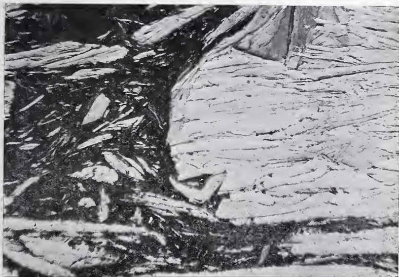
FIG. 10.—Cross section of Ceylon graphite grains embedded in clay, at a magnification of 133 diameters.
