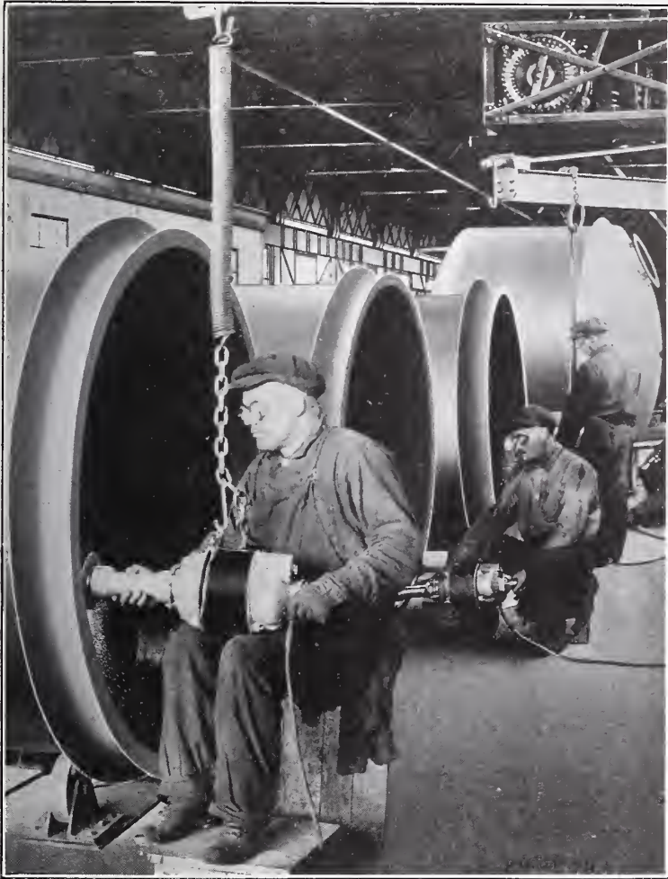
FIG. 3.—Grinding off weld.
