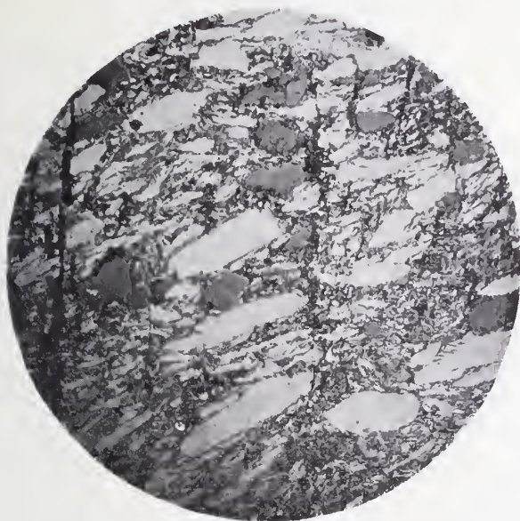
FIG. 23.—Cross section of a portion of a crucible wall in which the graphite is all Ceylon, \times 13.3 .
