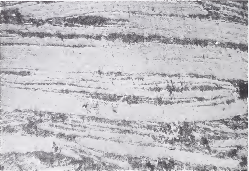
FIG. 8.—Cross section of Madagascar graphite flakes embedded in clay, at a magnification of 133 diameters.
