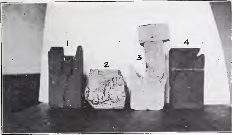
FIG 3.—Bricks after testing: (1) Magnesite. (2) Fire-clay. (3) Silica. (4) Chrome.
