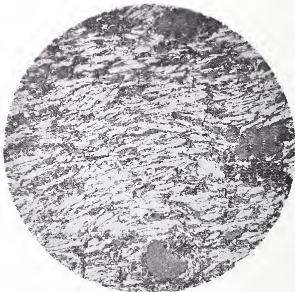
FIG. 20.—Cross section of a portion of a Japanese crucible wall, graphite unknown, \times 13.3 .
