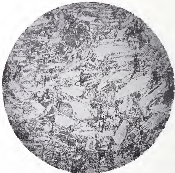
FIG. 30.—Cross section of a portion of a crucible wall in which 65% of the total graphite is Ceylon, 20% Alabama flake and 15% Madagascar flake, \times 13.3 .
