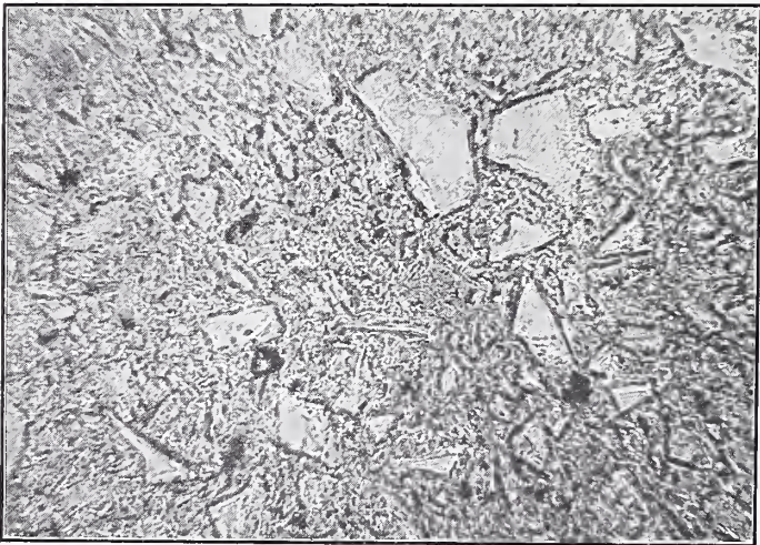
FIG. 2.—Five-hour burn, 1290° C. Sillimanite is still rather poorly developed. The quartz shows a beginning of solution by the rounding of the corners of the smallest grains. Magnification 300 diameters.
