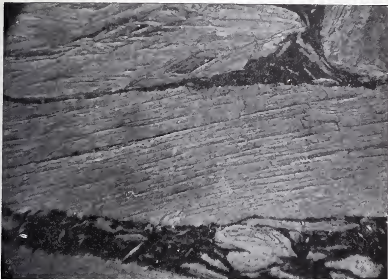
FIG. 9.—Cross section of Ceylon graphite grains embedded in clay, at a magnification of 133 diameters.
