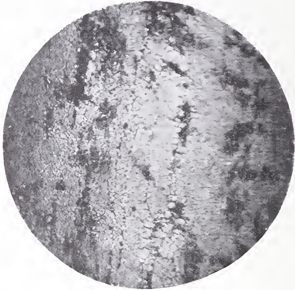
FIG. 17.—Cross section of a Madagascar graphite flake at a high magnification, \times 666 .
