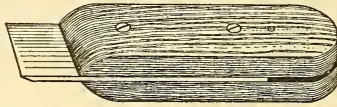
FIG. 78.—Knife for freezing microtome, made from the blade of a carpenter's plane.
