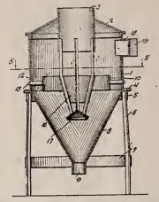
casing tangentially through the wall thereof, means suspended from the lower end of said outlet pipe for setting up an upwardly directed stream or current for discharge through the outlet pipe, and a tapered guide cylinder arranged between said air directing means and the outlet pipe having the upper end of greater diameter than the lower end thereof and arranged in alignment with said outlet pipe.
