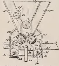
for the auxiliary hoppers, a receiver located beneath all of the hoppers and said coacting rollers, said receiver including a central compartment adapted to receive grain passing between said coacting rollers and further including laterally arranged troughs hav-ing conveyors therein, and scraper members bearing against said coacting rollers at the opposed portions thereof.
