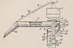
both sides of said pivotal mounting; a source of driv-ing power for said screw; and an automatically ad-justable driving shaft operatively connecting said con-veyor screw with said source of power at a point spaced from the pivotal mounting for the conveyor tube; whereby said conveyor may while in normal op-eration be adjusted horizontally or vertically within predetermined limits.
