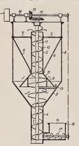
upper and lower ends, the lower portion of the con-duit and the adjacent portion of the screw being of greater radial dimension than the upper portions of these parts.
