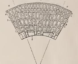
ribs of an adjacent series, and a plurality of series of substantially radially extending ribs on each sector so disposed that the radial ribs of one series will be in staggered relation with the ribs of an opposing similarly formed sector when said opposing sectors are in registry.
