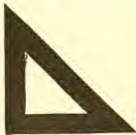
Fig. 109.—Open Hard Rubber Triangle, or Set-Square, 45, 45 and 90 degrees.
