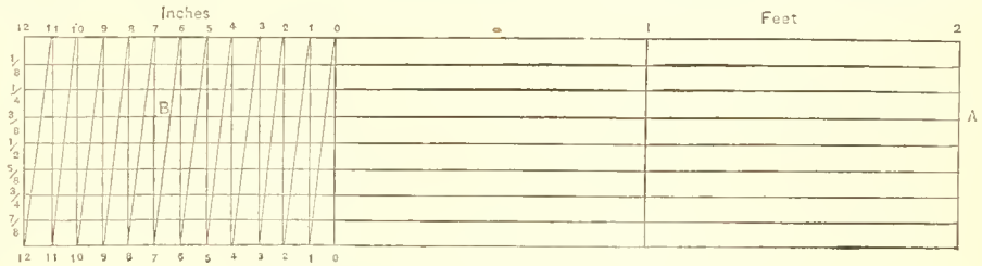
Fig. 121.—Diagonal Scale.— 1\frac{1}{2} inches to the foot.
