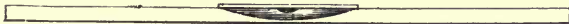
Longitudinal section of hollow-ground glass slide for observing bacteria in hanging drops.
