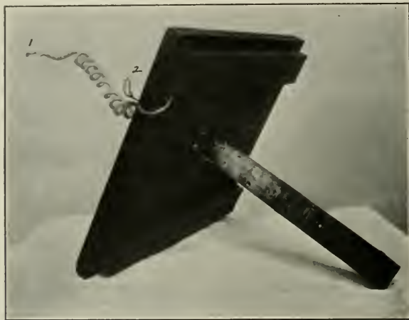
FIG. 179.—Interrupter Board with Lead and Glass Tube attached. The spiral wire, 1, is attached to the lead pipe. The loop, 2, is attached to the platinum wire. A slot is cut in the lead pipe close to the board for the outlet of the glass tube, which is inside the lead pipe. The latter is 12 inches long, with an inside diameter of 1\frac{1}{2} inches. Liquid in stone crock comes to within one inch of outlet of glass tube. (Original.)
