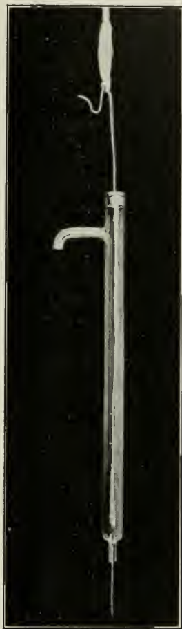
FIG. 180.—Interrupter tube. Length, 10½ inches; inside diameter, ½ inch. To the larger tube is sealed a capillary tube, 1½ inch long, through which a platinum wire slides. This capillary tube is large enough to carry the platinum wire without friction. (Original.)
