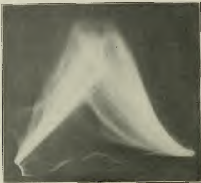
FIG. 178.—Illustrates flaming discharge, 8 inches in length. Meter will read 10 milliamperes with 10 amperes on primary circuit. Exposure for hip, in an adult weighing 160 lbs., 20 to 40 seconds. (Original.)
