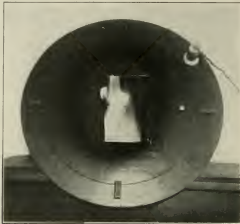
FIG. 176.—Illuminator. Light, evenly diffused, reflected from white back of box.
