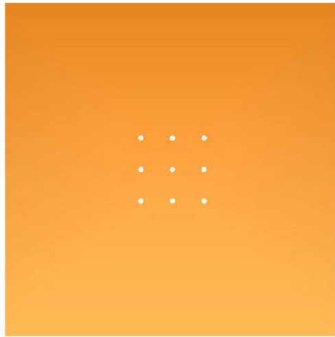
Figure 7. Copper-glass copper composite microstructure with 3x3 matrix of holes 10
