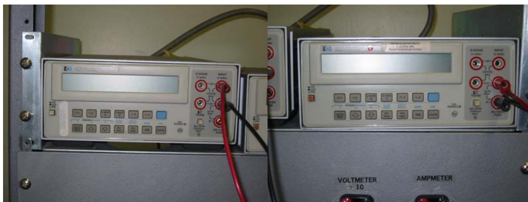
Figure 22. The voltmeter (left) and amp meter (right) used for the experiments
