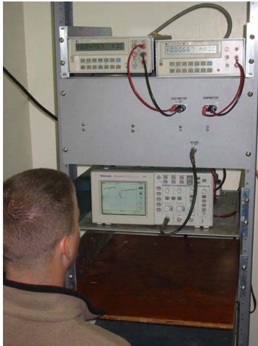
Figure 23. Jason Cooper recording the breakdown voltage on a sample
