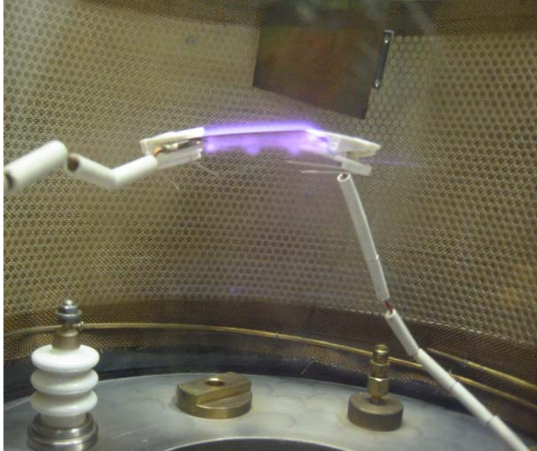
Figure 11. Glow discharge of sample after achieving breakdown voltage
