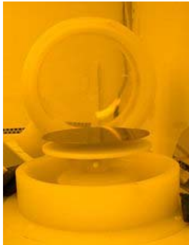
Figure 14. A spinner used to apply photo resist to the surface of a silicon wafer 17
