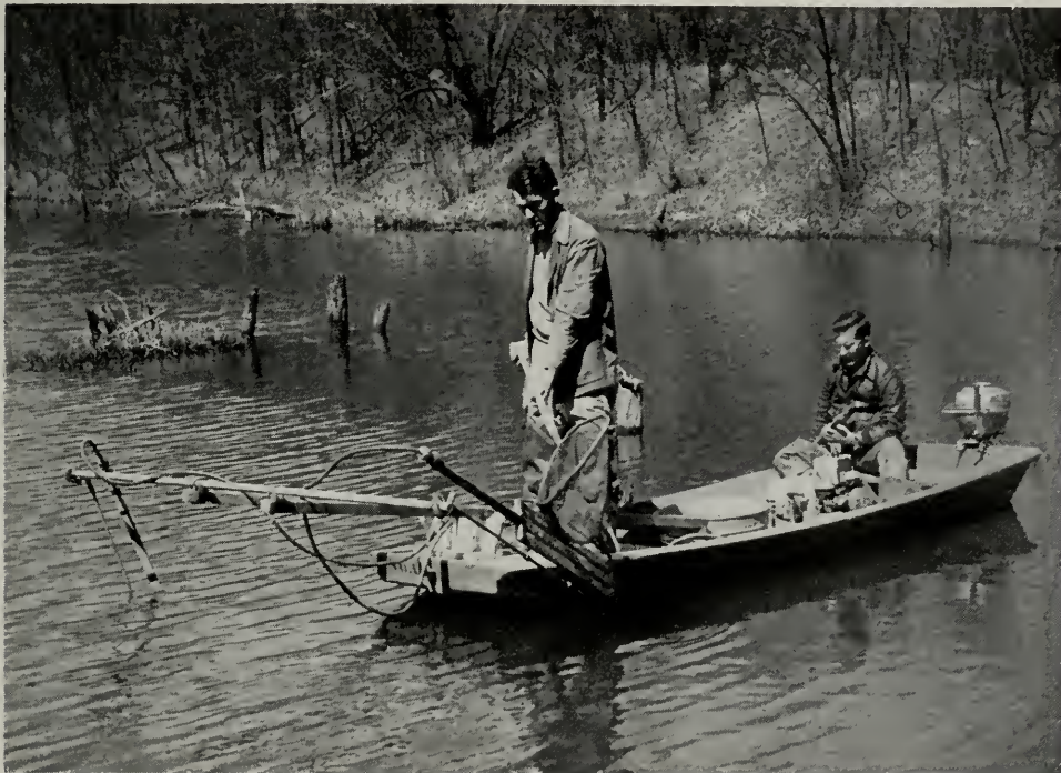
Fig. 5.—An electric fish shocker being used from a rowboat to collect warmouths in Park Pond.
