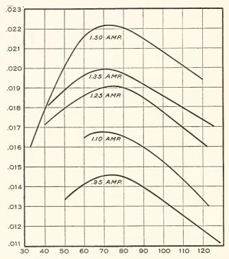
Fig. 14.—Calibration curves of ergometer II for magnetizing currents of 0.95 to 1.50 amperes.
