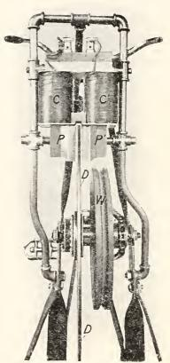
Fig. 2.—Electro-magnet and copper disk of ergometer 11. The copper disk D rotates in a magnetic field between pole-faces P and P'. Currents of varying strength are passed through coils C and C', thus varying the intensity of the magnetic field. The grooved wooden pulley W is used to drive the machine by a belt from a motor.
