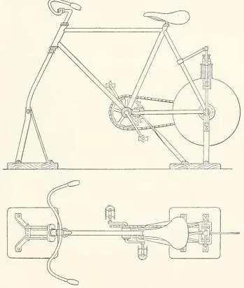
Fig. 1.—Side and top views of ergometer II.
