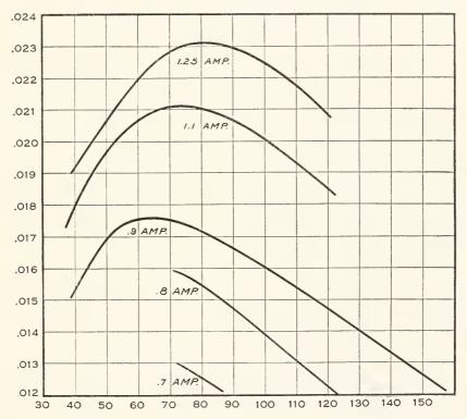
Fig. 8.—Calibration curves of ergometer 1 for magnetizing current of 0.7 to 1.25 amperes.
