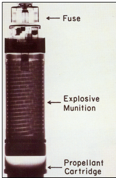
Fig. 1-59. This roentgenogram shows one of the rounds (the VOG-17) that the AGS-17 can fire, including its coil of notched wire, which is the source of the fragments. Note that the coiled wire and the explosive charge occupy about 75% of the rounds total volume.
