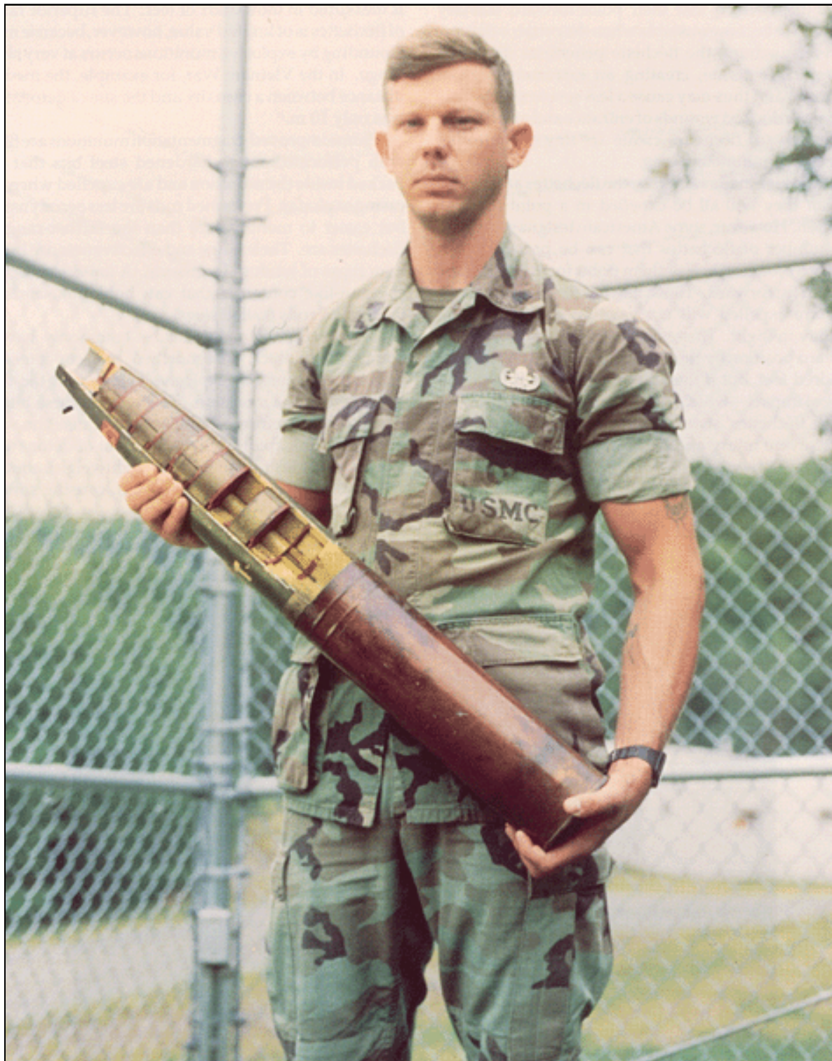
Fig. 1-29. The marine holds a cutaway demonstration model of a 105-mm improved-fragmentation munition (called a beehive round) that is loaded with flechette-filled containers. Source: Explosive Ordnance Disposal Group, Quantico Marine Corps Base, VA
