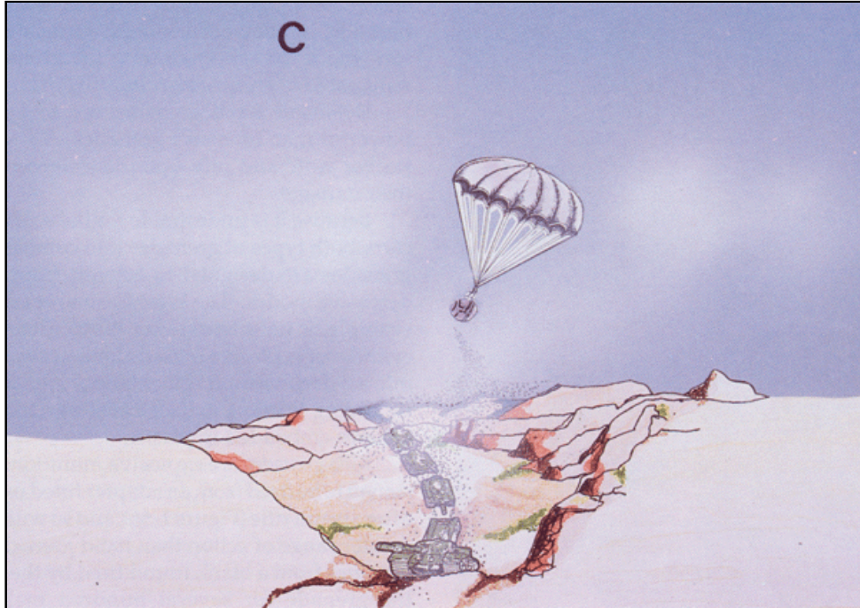
Fig. 1-53. The fuel mixes with the ambient air, forming an aerosol.
