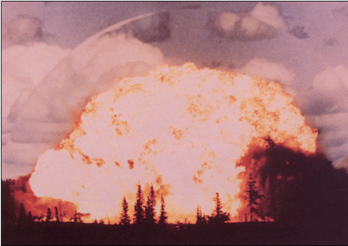
Fig. 7-1. A large conventional explosion is shown from a distance. Beyond the fireball, the blast wave appears as a sharp line, which is caused by refraction of light by the higher-density gas at the shock front.
