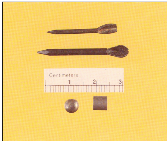
Fig. 1-27. These are typical preformed fragments. The smaller American-made flechette, which was extracted from a casualty, is bent and is missing a fin. Flechettes occasionally deform in tissue; such a deformation vastly increases their wounding potential. The smaller flechette weighs 550 mg; the larger Soviet-made flechette weighs 1.3 g. The ball and rod weigh 0.7 and 1.0 g, respectively.
