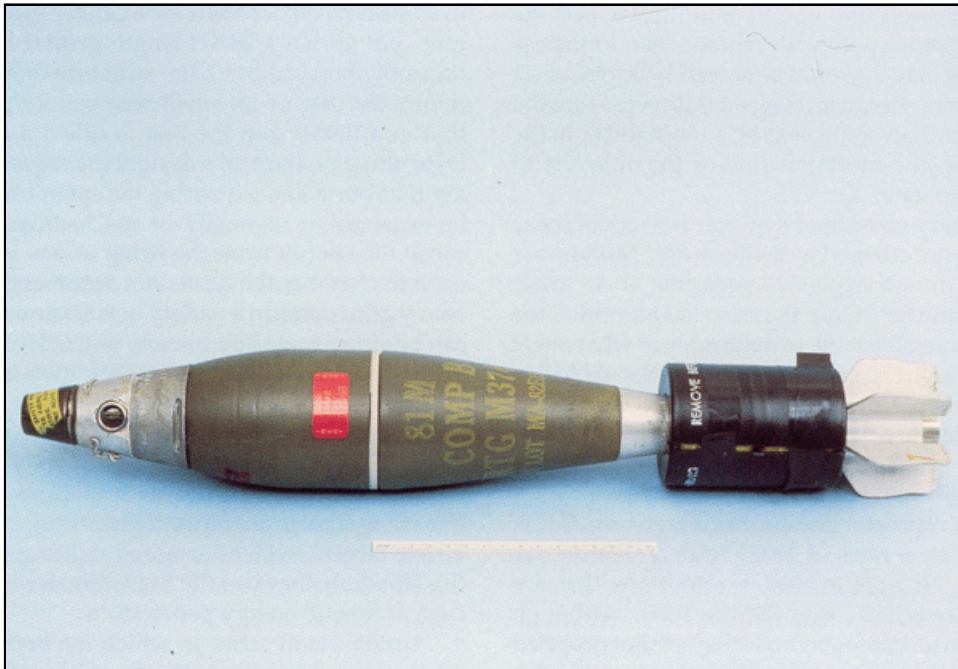
Fig. 1-47. The propellant of this 81-mm mortar bomb consists of (a) a shotgunlike cartridge within the tail and (b) an auxiliary charge, which is the black incremental-propellant container wrapped around the tail. The weight of the mortar bomb totals about 3.5 kg, one-third of which is the weight of the explosive charge. The controlled breakup of a prenotched metal coil under the thin external case creates fragments.
