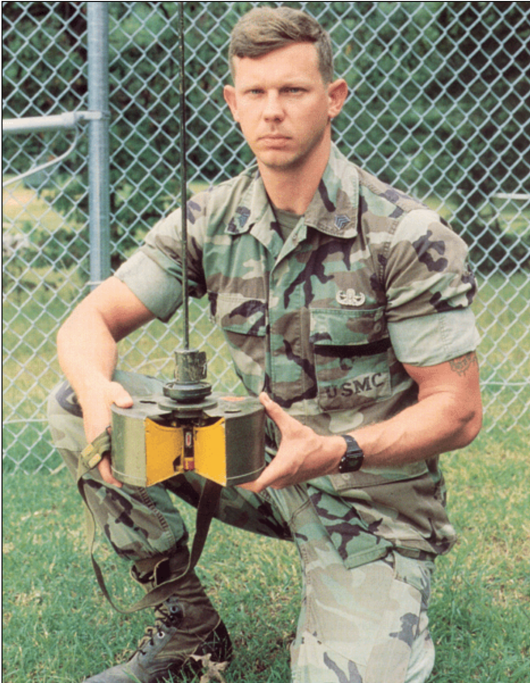
Fig. 1-64. This cutaway shows a portion of the 11-pound explosive charge (painted yellow) of an M21 antitank mine. The function of the thick concave melt plate that forms the upper margin of the explosive charge is similar in some respects to the melt sheet of a shaped-charge warhead. When the charge explodes, the metal plate breaks up into many high-velocity fragments that penetrate the tank and create far more damage than the blast alone would have done. The mine can be detonated either by a conventional pressure fuse that is activated by weight or a sophisticated tilt-rod extension fuse that is activated when the target vehicle's underside brushes it.
