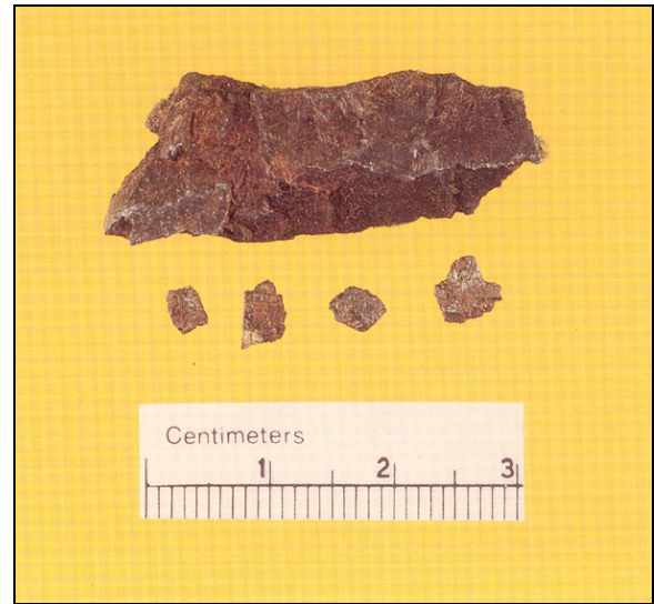
Fig. 1-25. These are random fragments. The larger chunk weighs 15.5g and is typical of the fragmentation munitions used in World War I; the smaller pieces weigh 100–200mg and are typical of those used in Vietnam.
