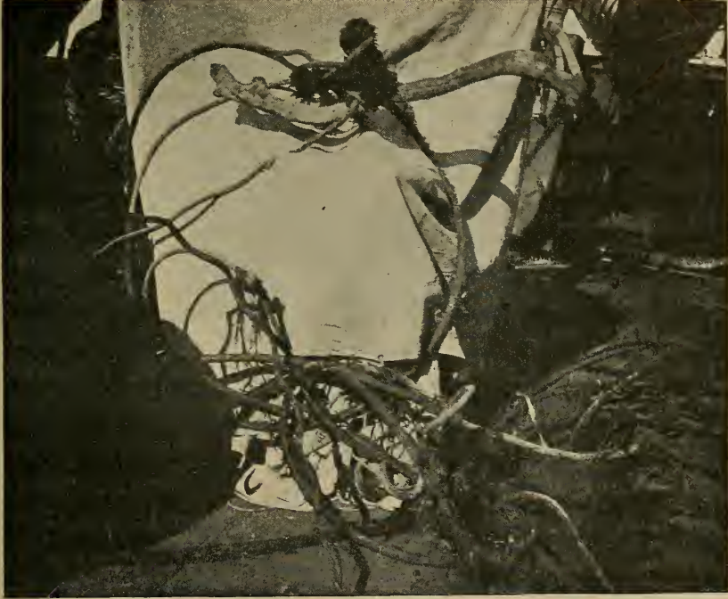
RECOVERED CABLE STRAND ENVELOPING BRANCH OF TREE
